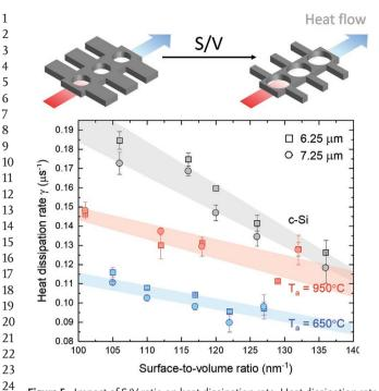
Figure 5. Impact of S/V ratio on heat dissipation rate. Heat dissipation rate  $\gamma$  as a function of the S/V ratio in nanobeams made of nc-Si with an average grain size of 163 ( $T_a = 650$  °C, blue), 215 nm ( $T_a = 950$  °C, red), and of single crystalline silicon c-Si (grey). Data is shown for two nanobeam lengths: 6.25 (squares) and 7.25 µm (circles). The colored stripes are guides to the eye.
