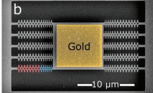
Figure 2. Structures for μ-TDTR measurements. a) SEM image of a suspended nc-Si membrane. b) SEM image of the nanobeams. The Bragg mirror of the bottom left beam is shown in red and half of the optomechanical cavity in blue. The central gold pad that is the transducer for μ-TDTR measurements is highlighted in yellow.
