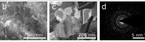
Figure 1. Structure of nanocrystalline silicon. a–c) Bright field planar TEM images of the nc-Si film with an average grain size of 215 nm and  $T_a = 950$  °C with increasing zoom, showing the randomly oriented grains and their relatively large size distribution. d) Selective area electron diffraction image.
