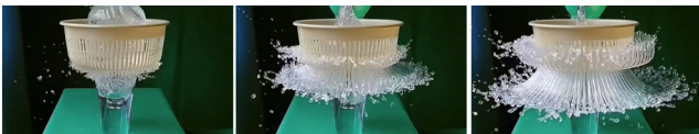
Fig. 20. Real colander. A real experiment of a water balloon being popped over a colander standing on a glass exhibits very similar features to what can be seen in Fig. 1 despite a different shape for the strainer: a two-crown splash appears as the water rushes through the interstices.
