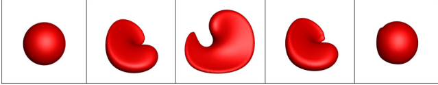
Fig. 10. Spherical interface in shear flow. We test our D3Q7 LBM-based integration of the phase field by passively advecting a spherical interface in a prescribed velocity field, see Eq. (29); snapshots obtained at t = 0 , t = T/4 , t = T/2 , t = 3T/4 , and t = T , from left to right.
