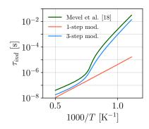
Figure 3:  $D-\kappa$  curves (left), and constant volume induction times,  $\tau_{\rm ind}$  (right) at  $\rho_{\rm vN}$  obtained with the modified simplified schemes compared with detailed kinetics results. Conditions: stoichiometric H<sub>2</sub>-O<sub>2</sub> at  $p_0=100$  KPa and  $T_0=300$  K.
