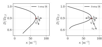
Figure 2: Influence of the thermodynamic and kinetic parameters on the calculated  $D - \kappa$  curves for single-step (left) and three-step chain-branching kinetics (right). The size of the arrows indicates how sensitive the curve is to changes in each parameter.
