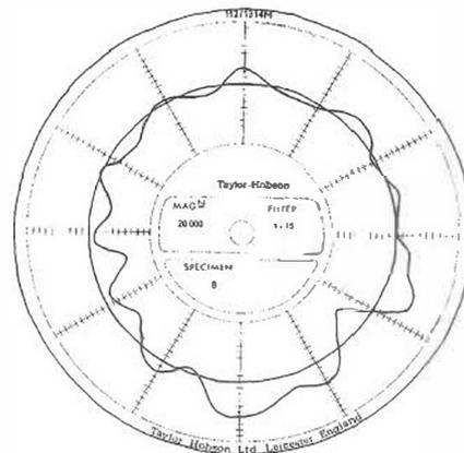
Fig 8. Flatness measurement on the rough surface B1
