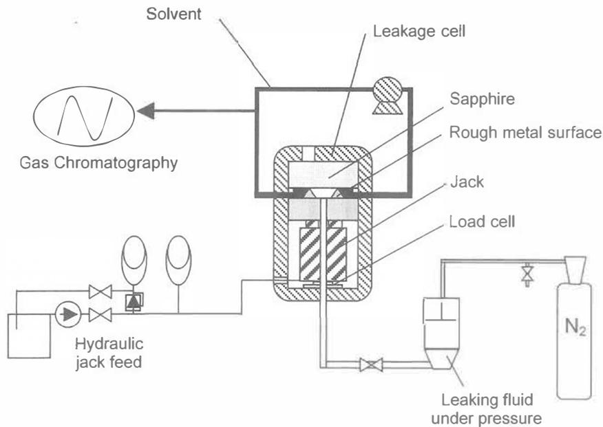
Fig 2. Description of the experimental apparatus
