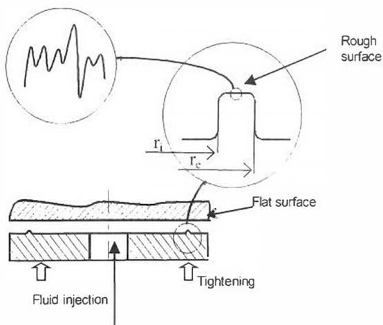
Fig 1. Configuration of the contact under study
