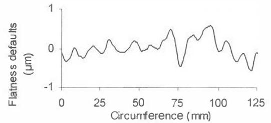
Fig 10. Cartesian representation of flatness measurement of figure 8
