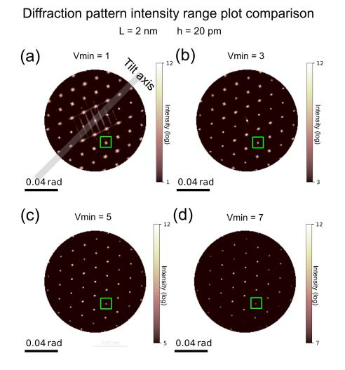
FIG. SI3: Different minimum log intensity plot comparison of corrugated WS<sub>2</sub> monolayer simulated diffraction pattern, where L = 2 nm and h = 20 pm. (a), (b), (c) and (d) are same simulation plot with  $V_{min}$ = 1, 3, 5, 7, respectively.
