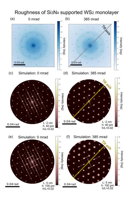
FIG. SI5: Roughness of  $Si_3N_4$  supported WS<sub>2</sub> monolayer. (a) and (b) are experimental results of diffraction patterns at 0 and 385 mrad tilt angles. (c) and (d) are the simulation results of h/L = 0.02 with period of L = 2 nm. (e) and (f) are the simulation results of h/L = 0.02 with period of L = 5 nm.
