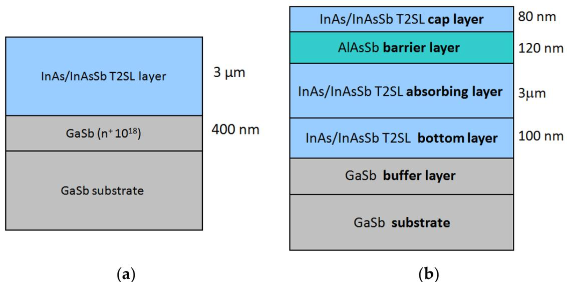
**Figure 1.** Schematic view of the different epilayers stacking under study. (a) T2SL structure used for absorption and photoluminescence measurements. (b) XBn detector structure used for lifetime, dark current, capacitance–voltage and quantum efficiency measurements.
