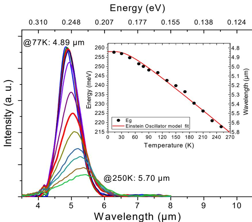
Figure 3. PL spectra of the Ga-free InAs/InAs<sub>0.63</sub>Sb<sub>0.37</sub> T2SL structure between 28 K and 250 K. Inset shows the temperature dependence of the T2SL’s bandgap where the solid line is a fit curve using Einstein oscillator’s equation.
