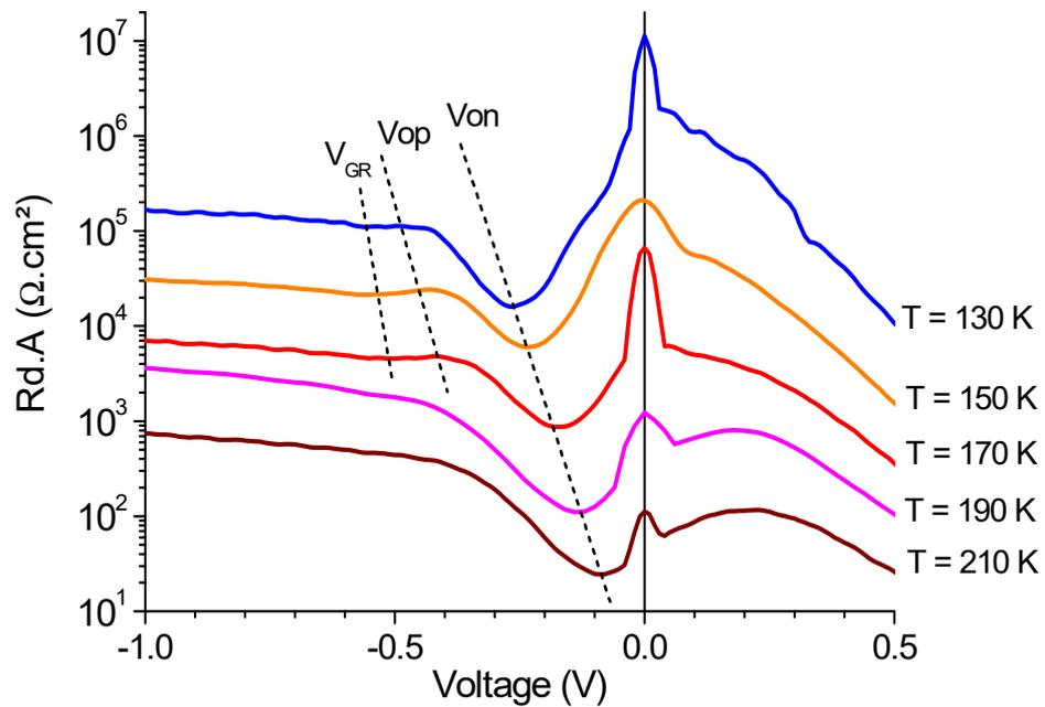
**Figure 8.** Differential resistance area ( $R_dA$ ) product as a function of the voltage for various detectors' temperature. Positions of relevant voltages ( $V_{on}$ ,  $V_{op}$ ,  $V_{GR}$ ) are identified (dotted line).
