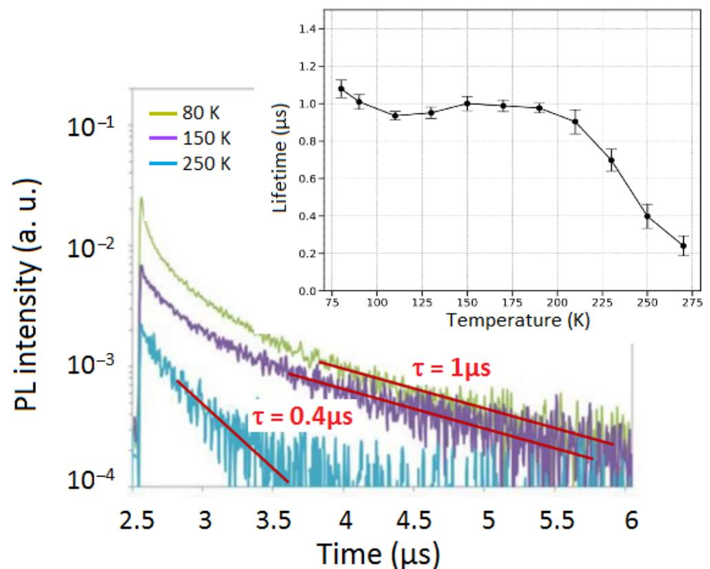
**Figure 4.** TRPL signal of the Ga-free XBn InAs/InAs<sub>0.63</sub>Sb<sub>0.37</sub> T2SL structure at 80 K, 150 K and 250 K. Inset shows the minority carrier lifetime values extracted from measurements.
