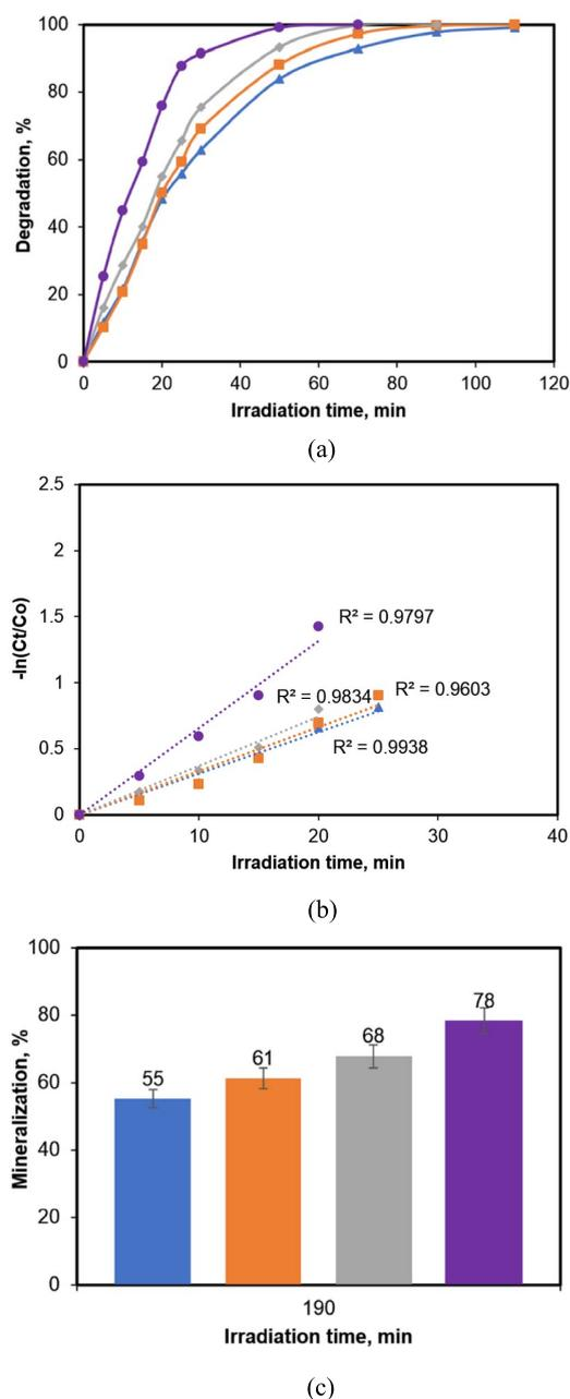
**Figure 5.** Influence of the pollutant concentration on the reaction performance. (a) Degradation yield; (b) pseudo-first-order kinetics; (c) mineralization yield (error bars represent standard deviation from duplicate experiment). (Photocatalyst dose 0.2 g/L) Regression equations:  $\blacktriangle$  25 mg/L ( $y = 0.0345x$ );  $\blacksquare$  15 mg/L ( $y = 0.0333x$ );  $\blacklozenge$  10 mg/L ( $y = 0.0372x$ );  $\bullet$  5 mg/L ( $y = 0.0659x$ ).
