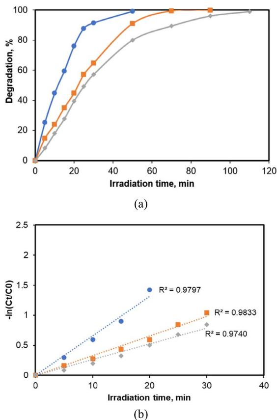
**Figure 7.** (a) Effect of inorganic ions on the CA degradation efficiency; (b) analysis of the experimental data for CA degradation according to pseudo-first-order kinetic model. ([CA] = 5 mg/L, 0.2 g/L photocatalyst). Regression equations: ● UPW ( $y = 0.0659x$ ); ■ Na<sub>2</sub>SO<sub>4</sub> ( $y = 0.0327x$ ); ◆ Na<sub>3</sub>PO<sub>4</sub> ( $y = 0.0263x$ ).
