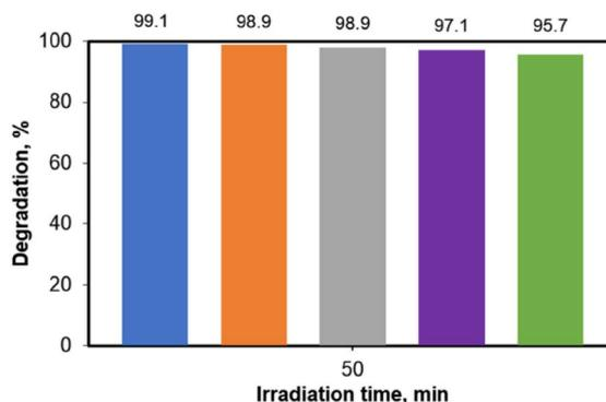
**Figure 8.** Performance of TiO<sub>2</sub>\_Pd photocatalyst over five consecutive working cycles in the photocatalytic degradation of CA ([CA] = 5 mg/L, 0.2 g/L photocatalyst).
