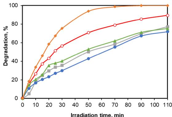
**Figure 1.** Photocatalytic activity of various TiO<sub>2</sub> photocatalysts (0.5 g/L) expressed as pollutant degradation efficiency (initial [CA] = 25 mg/L): ■ K7500; ● PC500; ○ TiO<sub>2</sub>; ▲ K7000; ◆ TiO<sub>2</sub>\_Pd.
