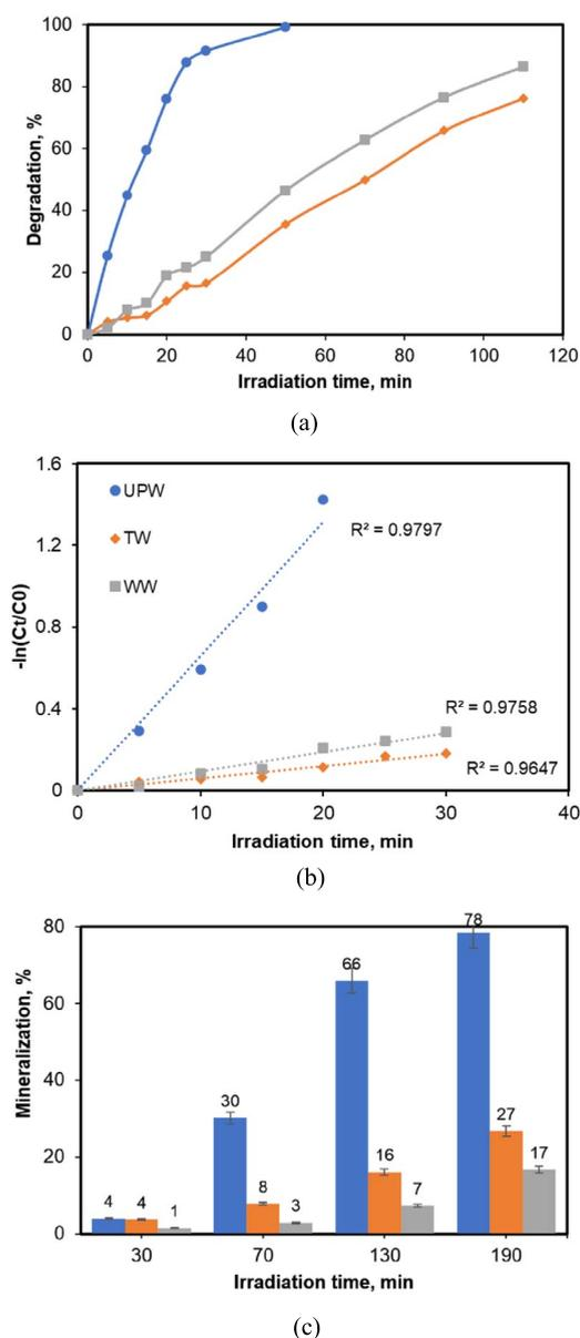
**Figure 6.** Effect of water matrix on CA degradation by TiO<sub>2</sub>\_Pd in the UV-A photocatalytic process. (a) Degradation efficiency; (b) analysis of the experimental data for CA degradation according to pseudo-first-order kinetic model; (c) mineralization (error bars represent standard deviation from duplicate experiment). ([CA] = 5 mg/L, 0.2 g/L photocatalyst). Regression equations: ● UPW ( $y = 0.0659x$ ); ◆ TW ( $y = 0.006x$ ); ■ WW ( $y = 0.0094x$ ).
