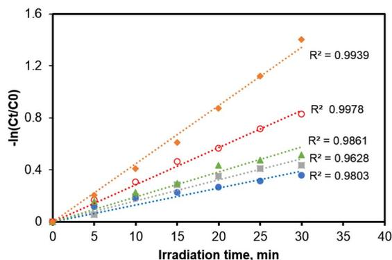
**Figure 2.** Pseudo-first-order kinetics deduced for the CA aqueous solution (25 mg/L) photodegradation in the presence of various photocatalysts (0.5 g/L dose). Regression equations: ■ K7500 ( $y = 0.0162x$ ); ● PC500 ( $y = 0.0131x$ ); ○ TiO<sub>2</sub> ( $y = 0.0521x$ ); ▲ K7000 ( $y = 0.0192x$ ); ◆ TiO<sub>2</sub>\_Pd ( $y = 0.0448x$ ).
