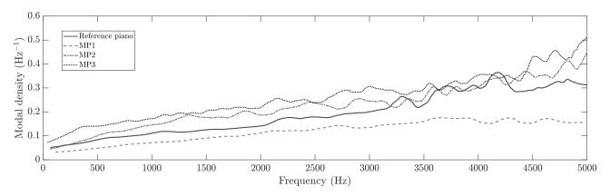
Figure 5. Modal density of the virtual soundboards as a function of the modal frequency.
