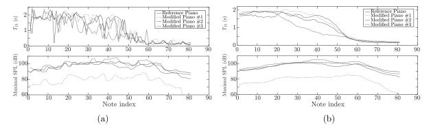
Figure 8. Energy decay time  $T_{15}$  (top) and maximal sound pressure level (bottom) computed from the simulated piano tones over the tessitura. Left (a) are the non-averaged features, and right (b) are the locally averaged features over an octave.
