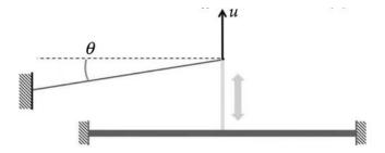
Figure 3. Figure and caption reproduced from Chabassier *et al.* [12]. Schematic view of strings-soundboard coupling at the bridge. The bridge is supposed to have a displacement u only along the vertical direction. The string forms a small angle  $\theta$  with the horizontal plane.
