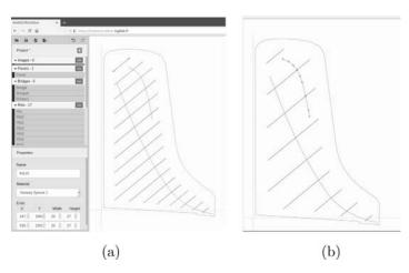
Figure 4. Screen shot of the GUI after completion of the design of the virtual Steinway D. The panel contour is shown in blue, the median line of the bridges in pink and the median lines of the ribs in green. Left (a) is the reference piano, right (b) is the modified piano 2, labeled as MP2
