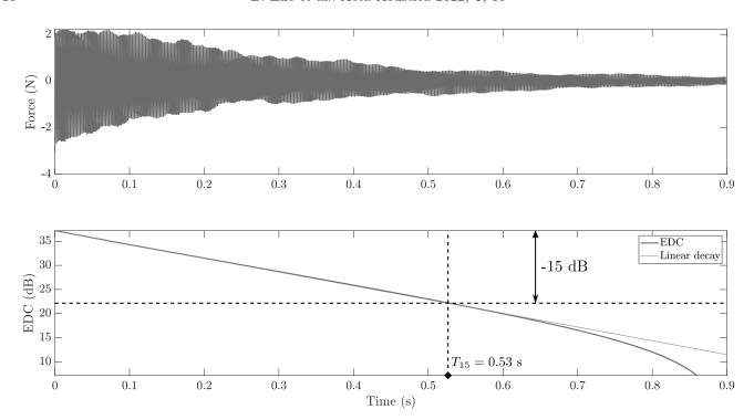
Figure 7. Example of energy decay curve (bottom) computed from the force applied by the A4 string to the soundboard of the reference piano (top). The linear part of the EDC (red solid line), obtained by linear interpolation, is used to compute the decay time  $T_{15}$ .
