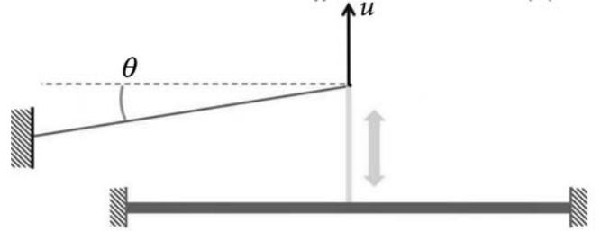
**Figure 3.** Figure and caption reproduced from Chabassier *et al.* [12]. Schematic view of strings-soundboard coupling at the bridge. The bridge is supposed to have a displacement  $u$  only along the vertical direction. The string forms a small angle  $\theta$  with the horizontal plane.
