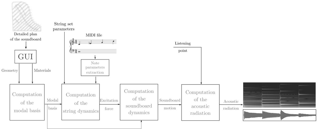
**Figure 1.** Block-diagram of the software architecture. The input data provided by the user are represented by a black font color. Blue corresponds to user data entered in the GUI. The software operations and the software outputs are represented by the red and green font colors, respectively.
