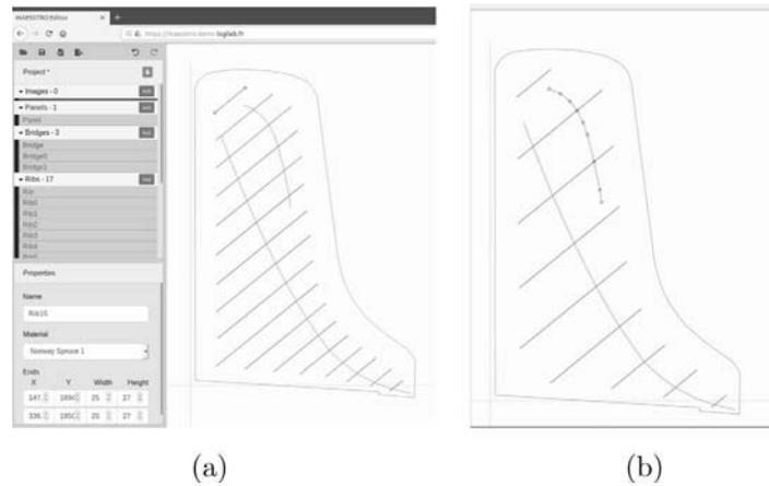
**Figure 4.** Screen shot of the GUI after completion of the design of the virtual Steinway D. The panel contour is shown in blue, the median line of the bridges in pink and the median lines of the ribs in green. Left (a) is the reference piano, right (b) is the modified piano 2, labeled as MP2
