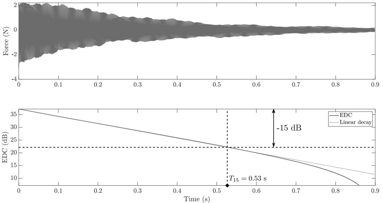
**Figure 7.** Example of energy decay curve (bottom) computed from the force applied by the A4 string to the soundboard of the reference piano (top). The linear part of the EDC (red solid line), obtained by linear interpolation, is used to compute the decay time  $T_{15}$ .
