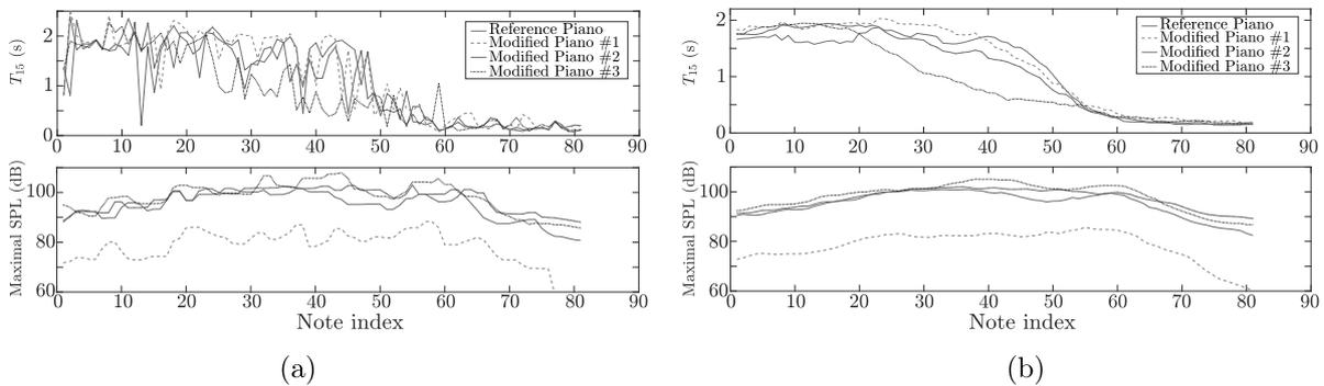
**Figure 8.** Energy decay time  $T_{15}$  (top) and maximal sound pressure level (bottom) computed from the simulated piano tones over the tessitura. Left (a) are the non-averaged features, and right (b) are the locally averaged features over an octave.
