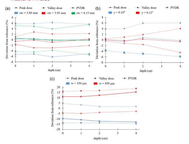
FIGURE 4 FIGURE 4 Variation in peak-to-valley dose ratios (PVDRs) and peak and valley doses with respect to the reference scenario as a function of depth and (a) center-to-center (c-t-c) distance, (b) slit divergence (γ), and (c) slit width (w)
