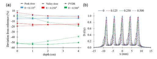
FIGURE 2 FIGURE 2 (a) Variation in peak-to-valley dose ratios (PVDRs), and peak and valley doses with respect to the reference scenario as a function of the collimator tilt (θ). (b) Lateral dose profiles at a 1 cm depth in water for different collimator tilts with respect to the beamline. The results based on Monte Carlo (MC) simulations
