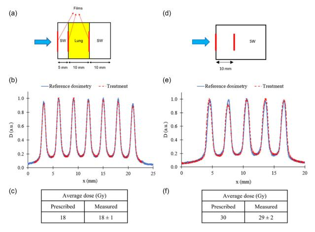
**FIGURE 7 FIGURE 7** Schematic representation of the experimental setup for the reference dosimetry prior to preclinical lung and brain irradiations (a and d), a comparison of the relative dose profiles measured in the reference dosimetry and small animal irradiation (b and e), and a comparison of the absolute average dose prescribed and measured during the irradiation (c and f). The left and right panels correspond to mouse lung and rat brain irradiations, respectively
