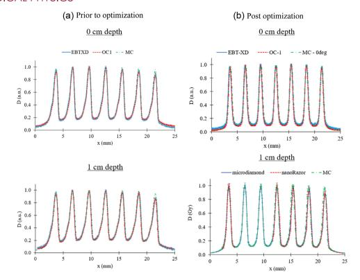
FIGURE 6 FIGURE 6 Lateral dose profiles at 0 and 1 cm depths in water (a) before and (b) after the beam alignment optimization. Dose profiles calculated by Monte Carlo (MC) codes and measured with EBT-XD and OC-1 films, and Razor and Microdiamond detectors are presented
