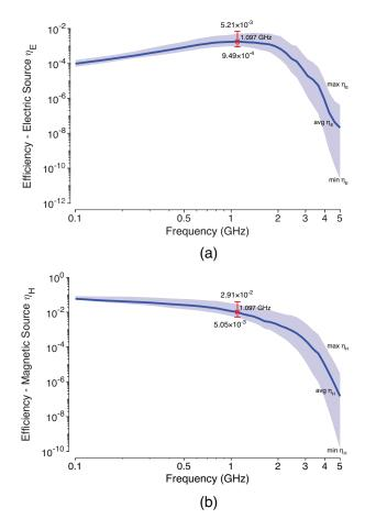
Fig. 3. Wireless power transfer efficiency for an (a) electric source and (b) magnetic source. The continuous blue line is the efficiency averaged (avg  $\eta$ ) over the 200 evaluated receiver positions. The upper and lower limits of the blue area represent the efficiency at the position that leads to the maximum (max  $\eta$ ) and minimum (min  $\eta$ ) values. The red bar indicates the variation in the efficiency at the optimal frequency.
