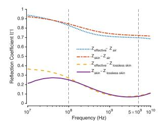
Fig. 2. Reflection coefficient for a plane wave propagating at the interface between two media for different scenarios. The wave impedance in the air is indicated as  $Z_{\rm air}$ , in the skin as  $Z_{\rm skin}$ , in the lossless skin as  $Z_{\rm lossless\,skin}$ , and  $Z_{\rm effective}$  in the effective medium composed of the nine tissues present in the pectoral model.
