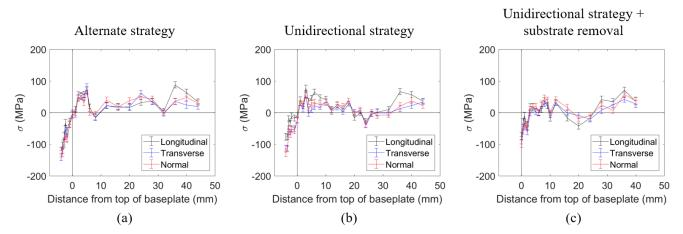
Figure 15: Evolution of the residual stresses along the height of the wall for each direction (longitudinal X, transverse Y and normal Z) within the samples built with (a) the alternate strategy; (b) the unidirectional strategy and (c) the unidirectional strategy after substrate removal.
