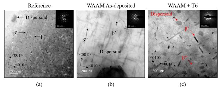
Figure 13: Bright-field TEM images of dispersoids, nanometric  $\beta$ '' and  $\beta$ ' phases and associated diffraction pattern for (a) the forged T6 material taken as the reference, (b) the WAAM as-deposited material and (c) the WAAM T6 material.
