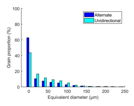
Figure 9: Grain size histogram obtained by EBSD
