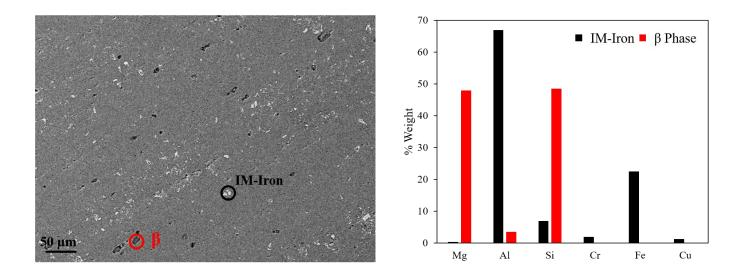
Figure 10: (a) SEM image with BSE contrast. (b) EDS of β-phase (red) and iron-IM (black).
