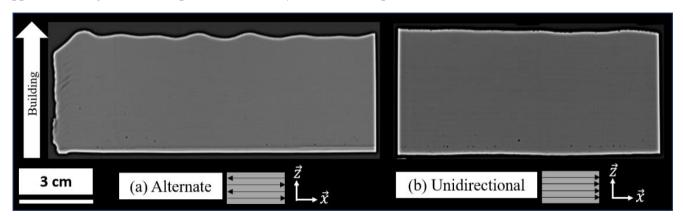
Figure 4 : X-Ray radiographs of the deposited walls (a) alternate strategy (b) unidirectional strategy.
