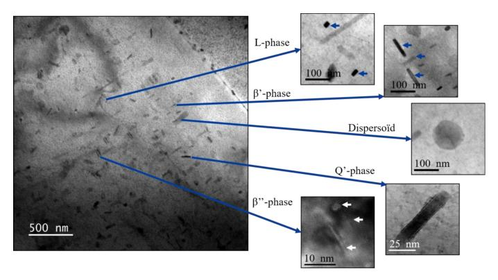
Figure 14: Bright-field TEM images of nanometric phases observed in the WAAM T6 material highlighting the presence of Q', L and β'' phases.
