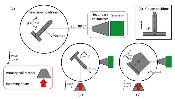
Figure 2: Schematic illustration of the set-up for neutron measurements (a) for transverse direction (Y); (b) for normal direction (Z); (c) for longitudinal direction (X); (d) gauge positions.
