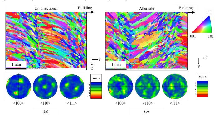
Figure 7: Grain morphology and crystallographic texture for the (a) unidirectional strategy and (b) alternate strategy.
