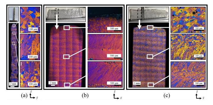
Figure 6: Macrographs illustration of the microstructure for the as-deposited WAAM AA6061 with magnification of enclosed regions by the white square for : (a) longitudinal section similar for both strategy, and in the X-Z plane section for (b) alternate strategy, (c) unidirectional strategy.
