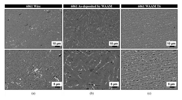
Figure 11: AA6061 at different metallurgical states (a) wire filler, (b) WAAM as-deposited material, (c) T6-treated WAAM material.
