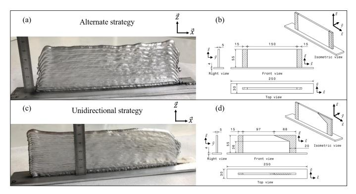
Figure 3: (a) geometry of the as deposited thin-wall for the alternate strategy; (b) final part geometry for the alternate strategy; (c) geometry of the as deposited thin-wall for the unidirectional strategy; (d) final part geometry for the unidirectional strategy.
