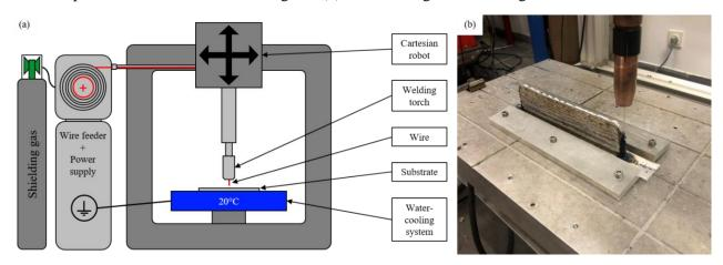
Figure 1: (a) Schematic experimental set up for deposition. (b) details of base plate clamping and cooling devices.
