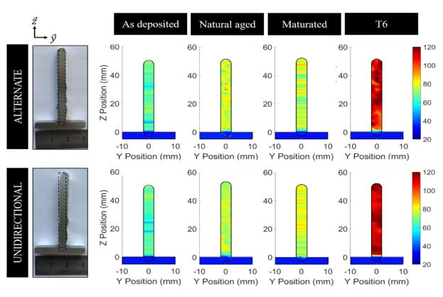
Figure 5: Hardness mapping for the two strategies and different metallurgical states
