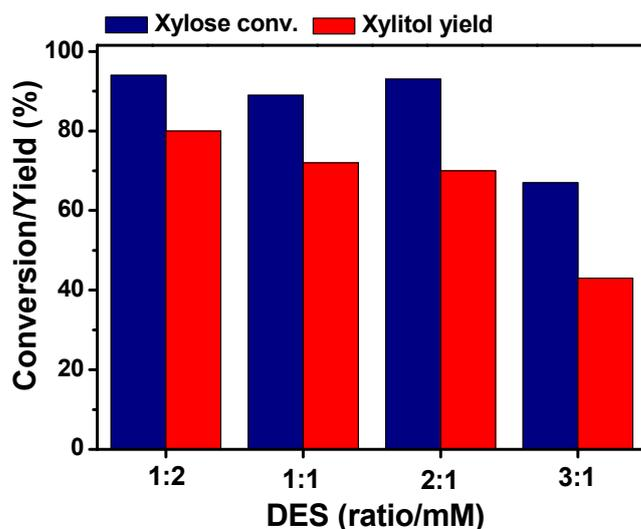
Figure 2. Effect of composition of DES components (reaction conditions: 1.5 g of DES, 0.5 mL of H<sub>2</sub>O, cat. 70 mg, H<sub>2</sub> = 30 bar, T = 110 °C, 3 h).
