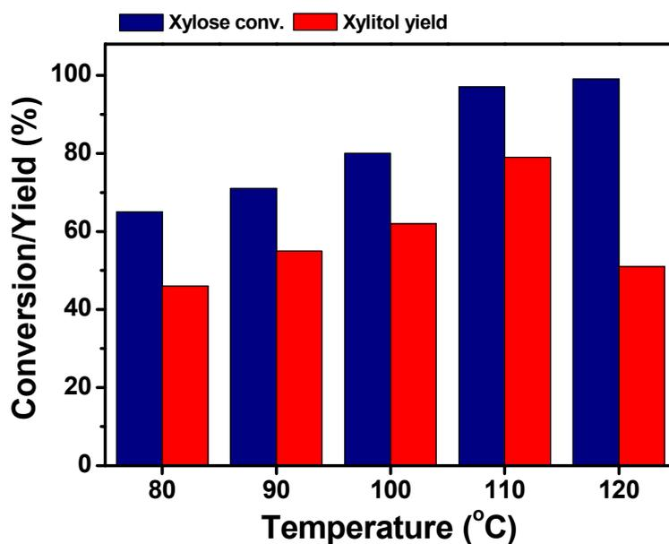
**Figure 4.** Effect of different temperature on DES phase reaction (reaction conditions: cat. 70 mg, 1.5 g of DES<sub>(3:1)</sub>, 0.5 mL of solvent, H<sub>2</sub> = 30 bar, 3 h).
