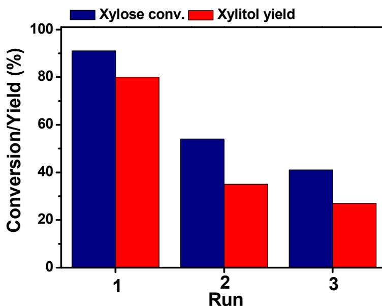
**Figure 5.** Recyclability potential of Ni<sub>3</sub>Fe<sub>1</sub> BMNPs in DES-phase catalytic hydrogenation of sugar (cat. 100 mg, DES<sub>(3:1)</sub>, H<sub>2</sub> = 30 bar, T = 110 °C, 3 h).
