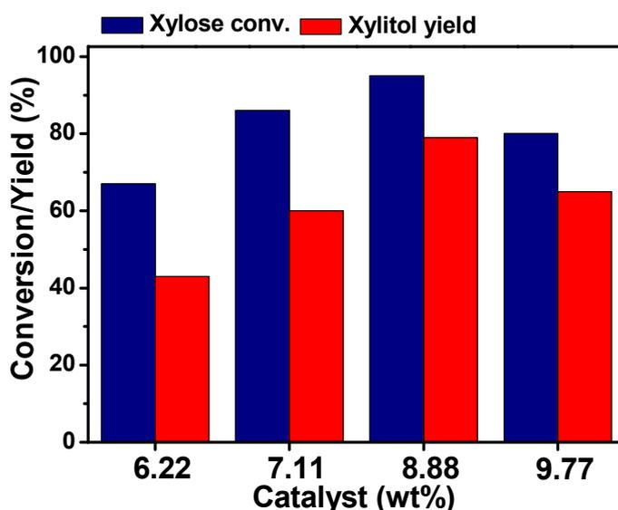
Figure 3. Effect of catalyst concentration/mass (reaction conditions: 1.5 g of DES<sub>(3:1)</sub>, H<sub>2</sub> = 30 bar, T = 110 °C, 3 h).
