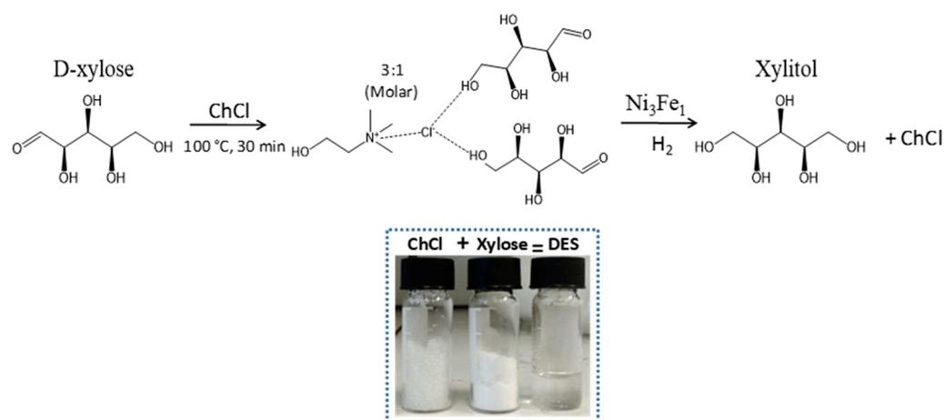
**Scheme 1.** DES phase hydrogenation of D-xylose into Xylitol.
