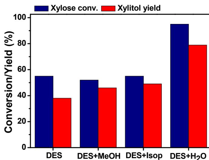
**Figure 1.** Effect of different solvents in DES phase reaction (reaction conditions: cat. 70 mg, 1.5 g of DES<sub>(1:2)</sub>, 0.5 mL of solvent, H<sub>2</sub> = 30 bar, T = 110 °C, 3 h).
