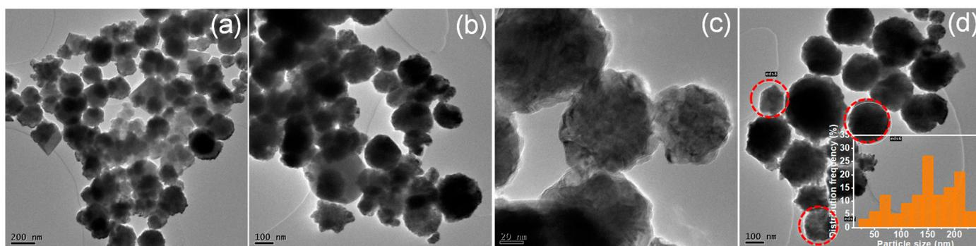
**Figure 6.** (a–d) Microscopic analysis (TEM) of fresh  $\text{Ni}_3\text{Fe}_1$  BMNPs at different magnification and inset (d) particle size distribution histogram of  $\text{Ni}_3\text{Fe}_1$  BMNPs.
