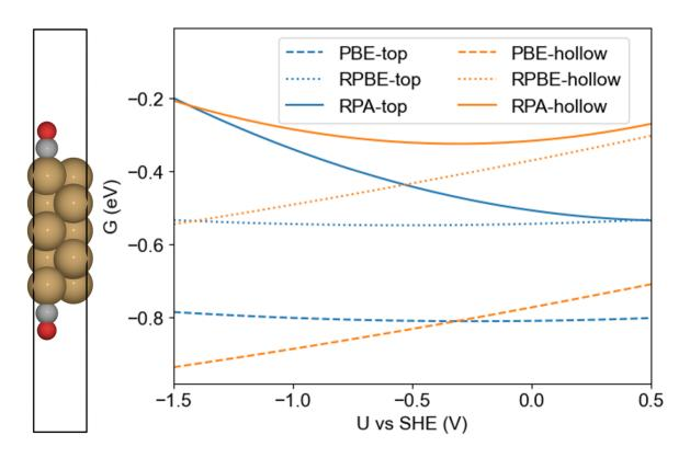
Figure 3: Potential dependent energetics of CO adsorbed at top (blue) and hollow (orange) site, using the grand canonical treatment with the PBE (dashed line), RPBE functionals (dotted line), and RPA (solid line). The experimentally inferred  $\sqrt{2} \times \sqrt{2}$  structure, where half of atop sites are covered by CO, is shown. Cu atoms are shown as brown, O atoms red, and C atoms grey.
