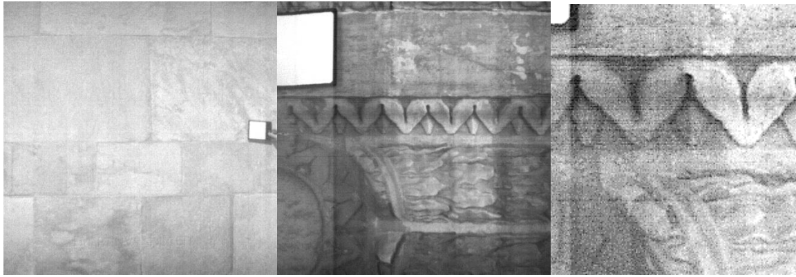
Figure 8: Comparison of the spectral images taken with the IQ camera at 1000nm on the marbles of the Pisa cathedral in (a) direct solar illumination; (b) indirect illumination. Figure (c) shows a detail of the structured noise affecting all the spectral region from 900 to 1000 nm.
