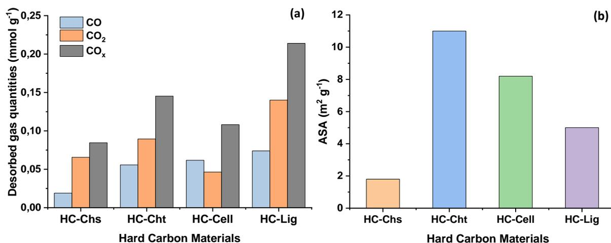
**Figure 5:** (a) Desorbed amounts of CO, CO<sub>2</sub> and CO<sub>x</sub> (CO + CO<sub>2</sub>) gases released by thermal decomposition during the TPD-MS experiment and (b) the active surface area (ASA) of hard carbon materials.
