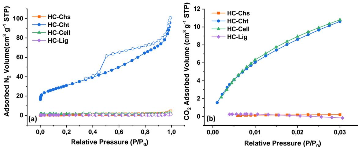
**Figure 3:** (a) Nitrogen adsorption/desorption isotherms measured at 77 K and (b) CO<sub>2</sub> adsorption isotherms measured at 273 K of HC materials: HC-Chs, HC-Cht, HC-Cell and HC-Lig.
