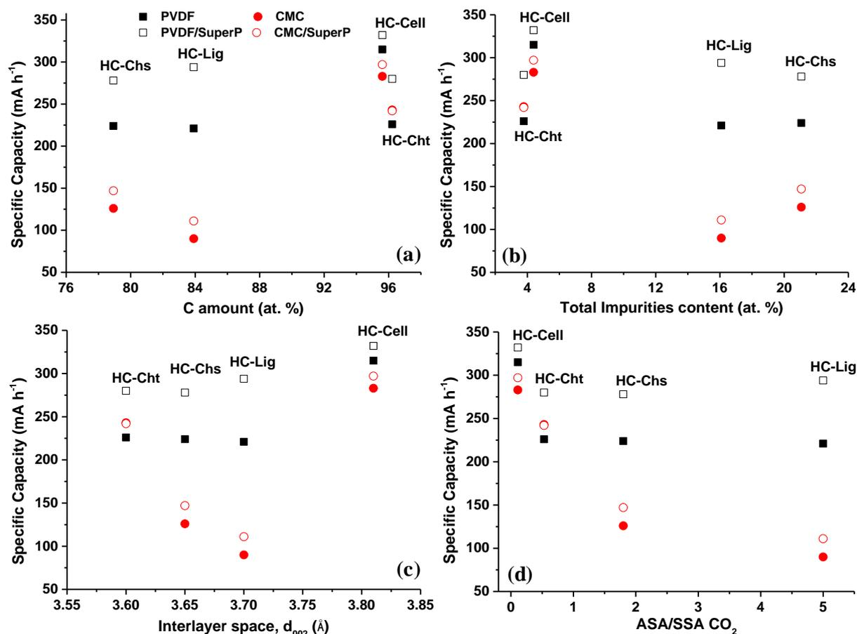
**Figure 10:** Correlation between the specific capacity and (a) the carbon amount (b) the level of impurities (including inorganic impurities, and oxygen- and other heteroatom-containing impurities detected by XPS), c) the interlayer spacing,  $d_{002}$ , and (d) the ratio of ASA to SSA CO<sub>2</sub>, for all four hard carbons formulated with PVDF and CMC binders without and with SuperP and tested in 1M NaPF<sub>6</sub> in EC:DEC.
