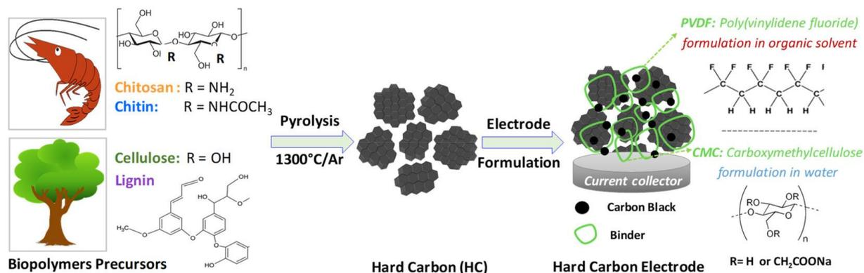
**Scheme 1:** Synthesis of hard carbon materials by pyrolysis of biopolymers and the electrode preparation.
