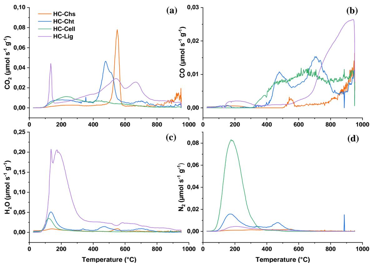
**Figure 4:** Gas desorption profiles of (a) CO<sub>2</sub>, (b) CO, (c) H<sub>2</sub>O and (d) N<sub>2</sub> obtained by TPD-MS for HC-Chs, HC-Cht, HC-Cell and HC-Lig hard carbons.
