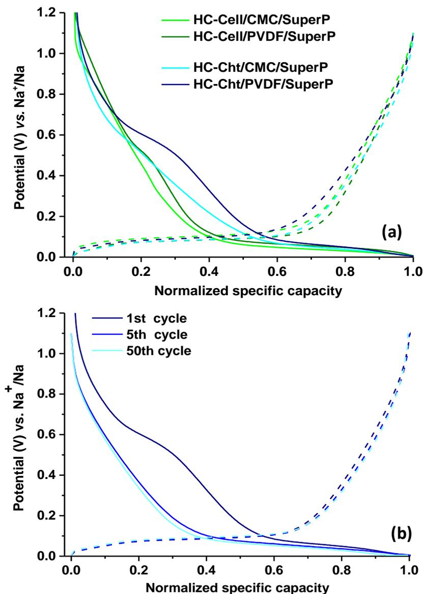
**Figure 7:** (a) 1<sup>st</sup> charge/discharge cycle for the cells assembled with HC-Cell and HC-Cht formulated with CMC /SuperP and PVDF /SuperP, and (b) the charge/discharge profiles of the 1<sup>st</sup>, 5<sup>th</sup> and 20<sup>th</sup> cycle for the HC-Cht PVDF/SuperP. These tests were performed using in 1 M NaPF<sub>6</sub> in EC:DEC as electrolyte.
