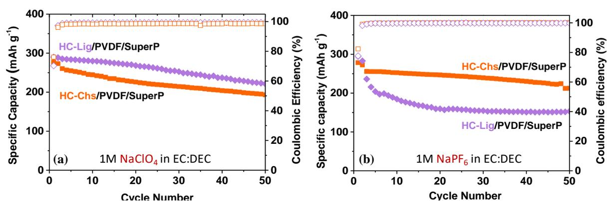
**Figure 8:** Specific capacity (full symbols) and Coulombic efficiency (empty symbols) of the Na-ion half-cells tested with electrodes based on HC-Lig and HC-Chs formulated with PVDF /SuperP, and (a) 1M NaClO<sub>4</sub> in EC:DEC and (b) in 1M NaPF<sub>6</sub> in EC:DEC.
