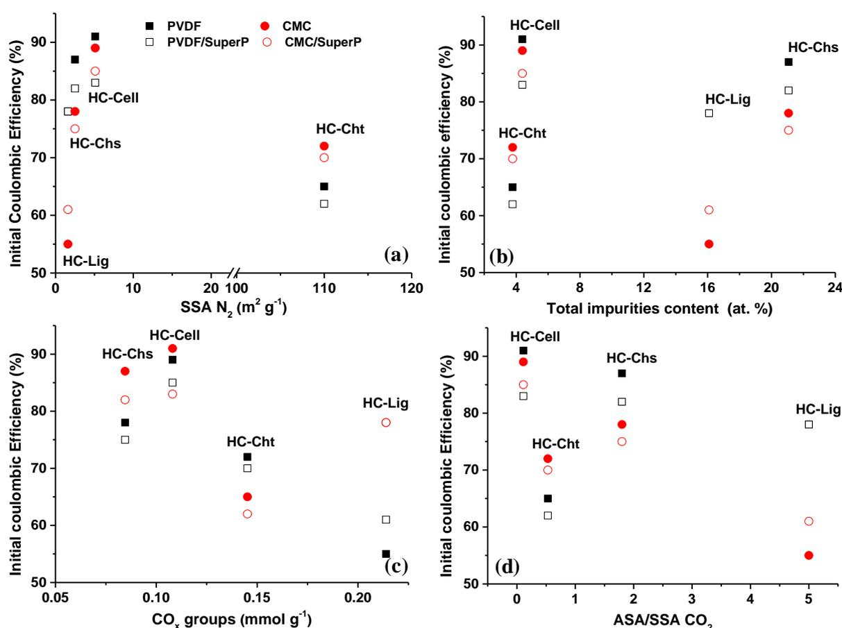
**Figure 9:** Correlation between the initial coulombic efficiency, iEC, and (a) the specific surface area, SSA N<sub>2</sub>, (b) the level of impurities (including inorganic impurities, oxygen- and other heteroatom-containing impurities detected by XPS), c) the oxygen-containing functional groups, CO<sub>x</sub> and (d) the ratio of ASA to SSA CO<sub>2</sub> for all four hard carbons formulated with PVDF and CMC binders without and with SuperP, and tested in 1M NaPF<sub>6</sub> in EC:DEC.
