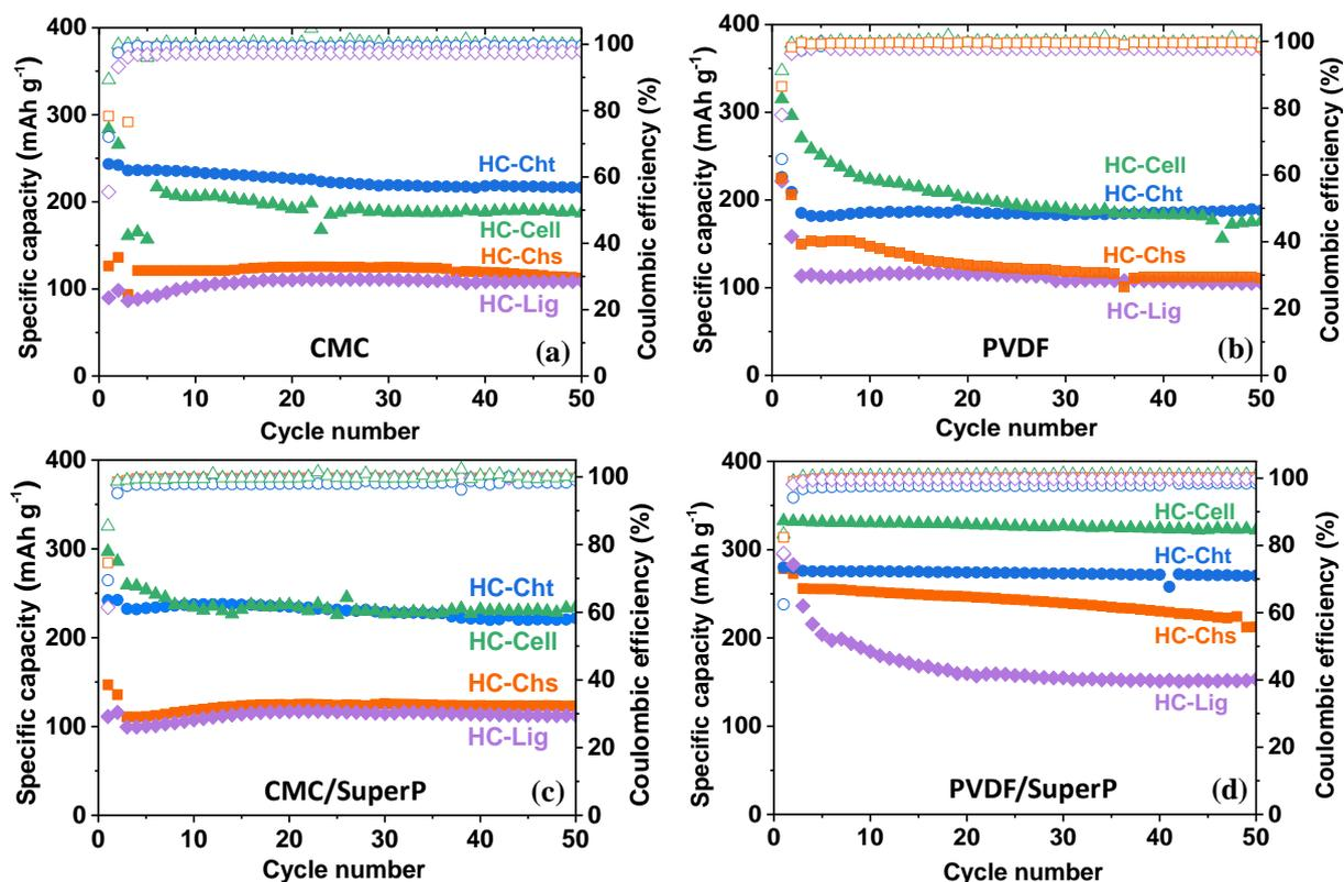
**Figure 6:** Specific charge capacity (full symbols) and Coulombic efficiency (empty symbols) of the Na-ion half-cells tested with electrodes based on four different HCs formulated with (a) CMC, (b) PVDF (c) CMC /Super P and (d) PVDF/SuperP binders in 1 M NaPF<sub>6</sub> in EC:DEC electrolyte. The first two cycles were performed at a rate of C/10. The rest of the cycling proceeded at a rate of C/5.
