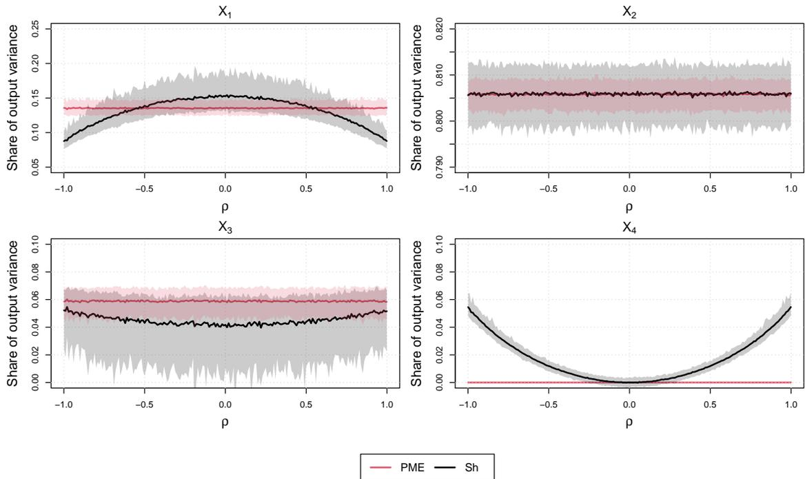
Figure 3: PME and Shapley effects for the Ishigami model with a spurious variable, with respect to the correlation coefficient  $\rho$  between  $X_1$  and  $X_4$ . The grey and red areas around the solid plots give the 95%-confidence intervals of the estimates.
