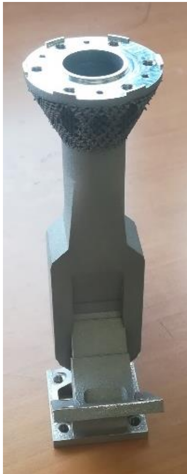
Fig. 8. Prototype of the 3D-printed Bøifot OMT in SLM using aluminium powder (AlSi10Mg).
