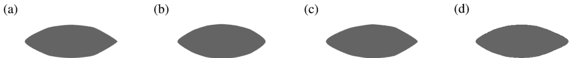
Figure 8: (a) Reference optimal shape for the minimum drag test case at Re = 1 with n_p = 5 control points and fixed inner curvature radius. (b) Same as (a) with n_p = 7 control points and fixed inner curvature radius. (c) Same as (a) with n_p = 5 control points and variable inner curvature radius. (d) Reference optimal shape discretized with n_p = 7 control points, after DRL has adjusted the end and inner curvature radii to restore the proper cross-sectional area.
