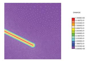
Figure 15: Modified edge-cracked plate. Damage distribution ( $l_c = 0.05 \, mm$ ).
