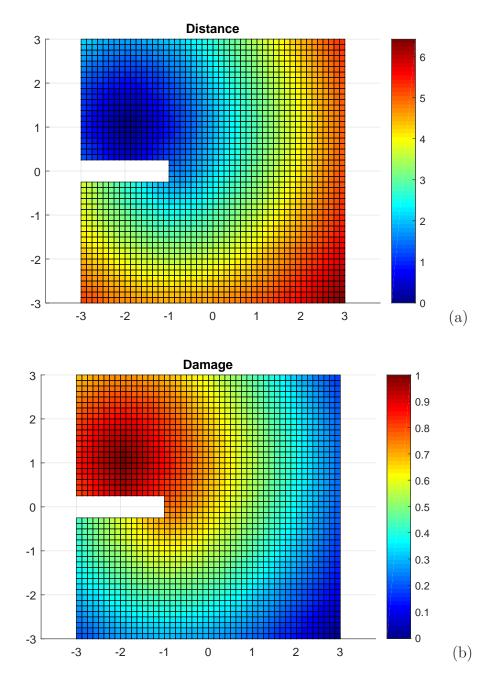
Figure 2: Level set (a) and damage field (b) on a notched plate.
