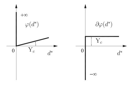
Figure 3: Dissipation function and its subdifferential.
