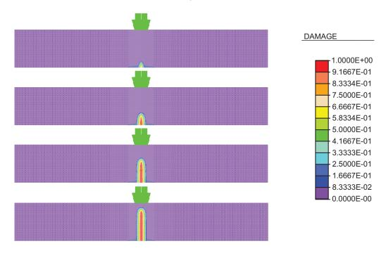
Figure 18: Three-point bending of a beam. Iso-damage maps showing damage evolution for  $l_c = 40.0 \, mm$ .
