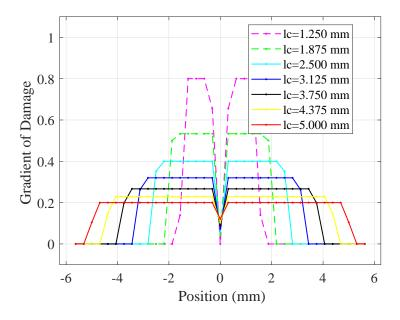
Figure 9: Imperfect bar in tension. Gradient of damage distribution at complete localization.
