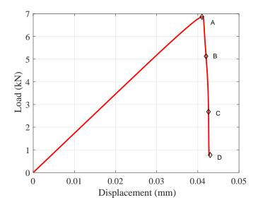
Figure 22: Asymmetric double-notched plate. Load-deflection curve.
