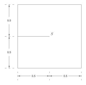
Figure 12: Edge-cracked plate. Model problem.
