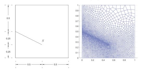
Figure 14: Modified edge-cracked plate. Model problem and FE mesh.
