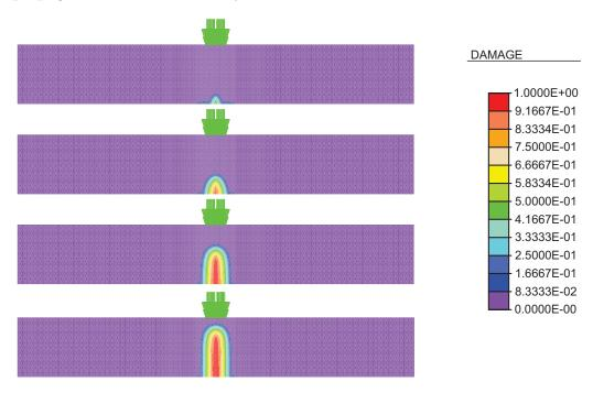
Figure 19: Three-point bending of a beam. Iso-damage maps showing damage evolution for  $l_c = 80.0 \, mm$ .
