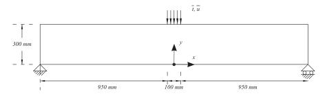
Figure 16: Three-point bending of a beam. Model problem.
