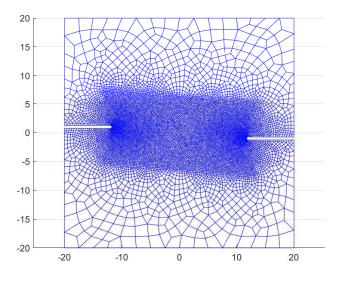
Figure 21: Asymmetric double-notched plate. FE mesh.
