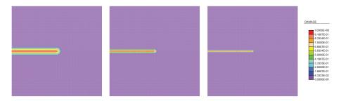
Figure 13: Edge-cracked plate. Damage distribution for different length scales  $l_c$  (from left to right:  $l_c = 0.05 \, mm$ ,  $l_c = 0.025 \, mm$ ,  $l_c = 0.0125 \, mm$ ). The thickness of the damaged region equals  $2 \, l_c$ .
