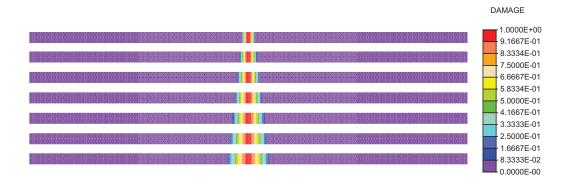
Figure 11: Imperfect bar in tension. Damage distribution at final stage of loading process for different length scales  $l_c$  (from top to bottom:  $l_c = 1.250 \, mm$ ,  $l_c = 1.875 \, mm$ ,  $l_c = 2.500 \, mm$ ,  $l_c = 3.125 \, mm$ ,  $l_c = 3.750 \, mm$ ,  $l_c = 4.375 \, mm$ ,  $l_c = 5.000 \, mm$ ).
