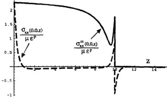
Fig. 2. Distributions of the original stress component  $\sigma_{xx}$  along the  $z$ -axis and of the surface stress  $\sigma_{xx}^m$  after matter removal of thickness  $z$ .
