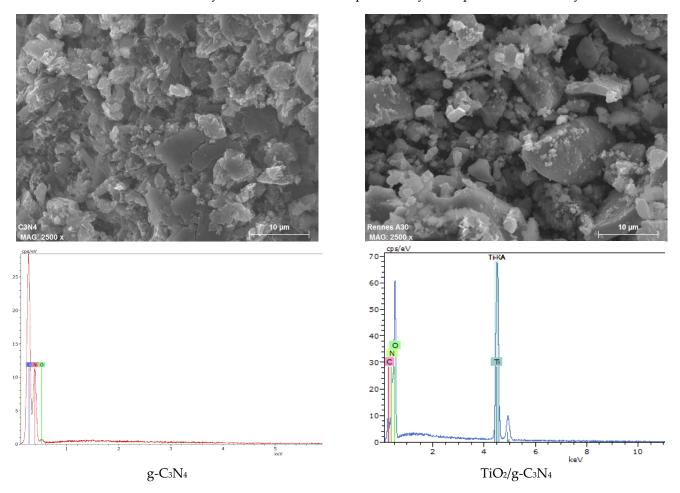
Figure 2. SEM images with EDX spectra of g-C3N4 and TiO<sub>2</sub>/g-C<sub>3</sub>N<sub>4</sub>.
