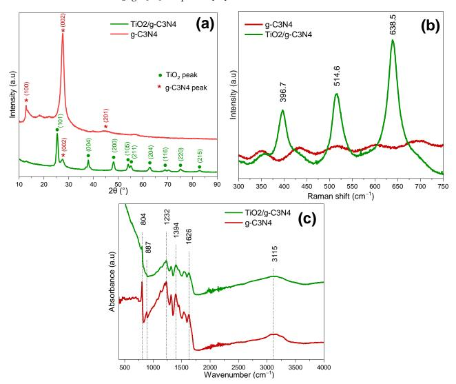
**Figure 3.** (a) XRD patterns of materials; (b) Raman spectra and (c) FTIR spectra of g- $C_3N_4$  and  $TiO_2/g$ - $C_3N_4$  composites.
