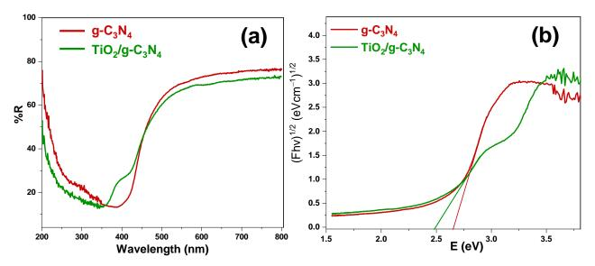
**Figure 4.** Diffuse Reflectance Spectra (**a**) and plot of transferred Kubelka-Munk versus energy of the light absorbed (**b**) of pure  $g-C_3N_4$  and  $TiO_2/g-C_3N_4$ .
