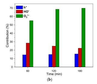
**Figure 14.** (a) Effect of additives in the degradation of 10 ppm of BPB and (b) Contribution of various active species in the photodegradation (500 mL of BPB solution, natural pH, under UV irradiation).
