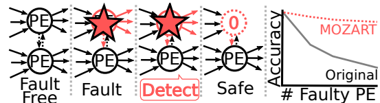
Fig. 1. MOZART Provides On-Line Testing and Fault Masking with Graceful Degradation in Accuracy
