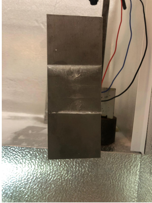
Figure 12 – Example of ice failure for a 44 mm-long ice block using the first flexural mode (200 V)
