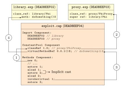
Fig. 3. BCV view when verifying exploit.cap file.
