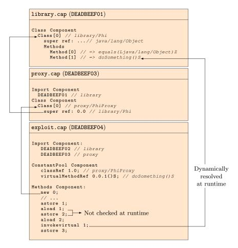
Fig. 4. Runtime view when executing exploit.cap.
