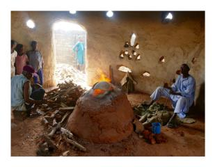
Fig. 4 Bikini furnace for production of raw glass, with bellows, bellows operator, and the worker who inserts firewood
