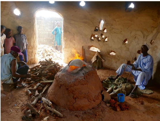
Fig. 4 Bikini furnace for production of raw glass, with bellows, bellows operator, and the worker who inserts firewood
