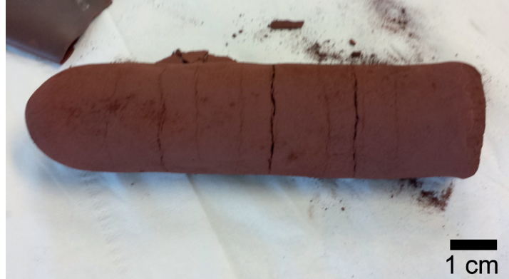
Fig. 3. Green-body moulded with a thick wall soft-bag. The cracks can be observed in the surface. These cracks are formed after the pressing, while reducing the isostatic pressure.
