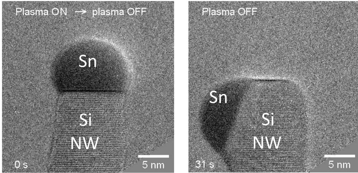
**Figure 1.** SiNW grown *in situ* in NanoMAX with Sn catalyst, at the moment of switching plasma off (0 s, left) and 31 s after plasma has been switched off (right).
