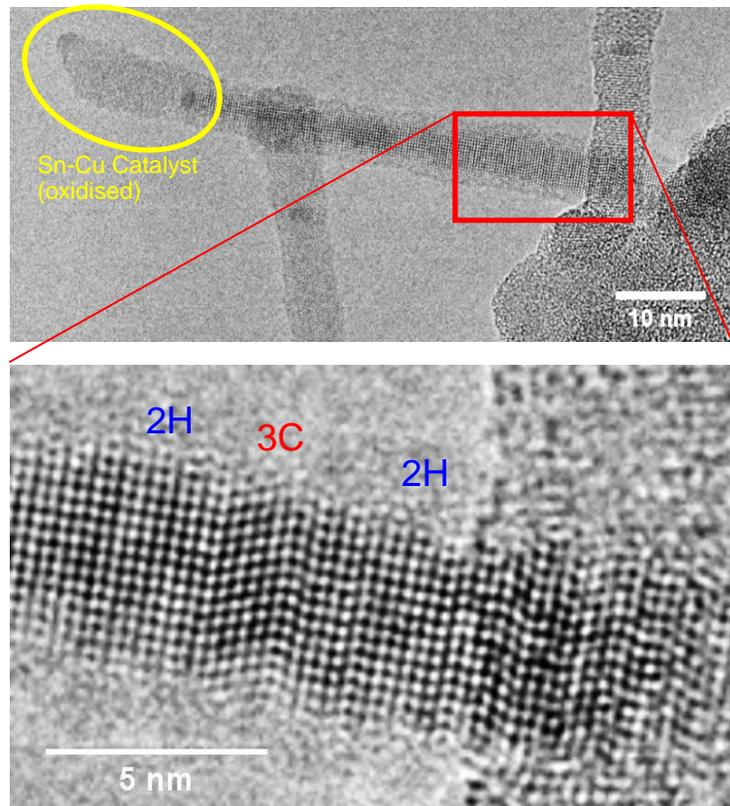
**Figure 2.** 2H SiNW obtained in a PECVD reactor [4], with a short 3C (cubic) domain.
