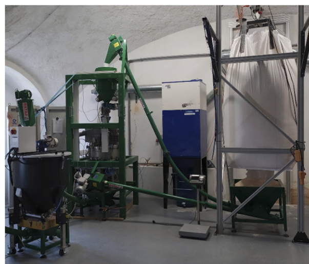
Figure 10. A low-pressure plasma reactor for the treatment of polymer powders.
