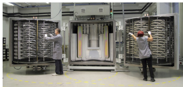
Figure 8. A low-pressure plasma reactor in a metallic chamber.
