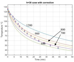
**Fig. 4.** Simulated coupling phase with specific heat varying from 600 to 1200J/kg.K. Comparison with measured data with error crosses ('+')
