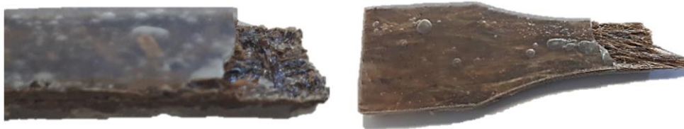
Figure 12. Visualization of fracture defects (delamination) on sandwich tensile specimens.
