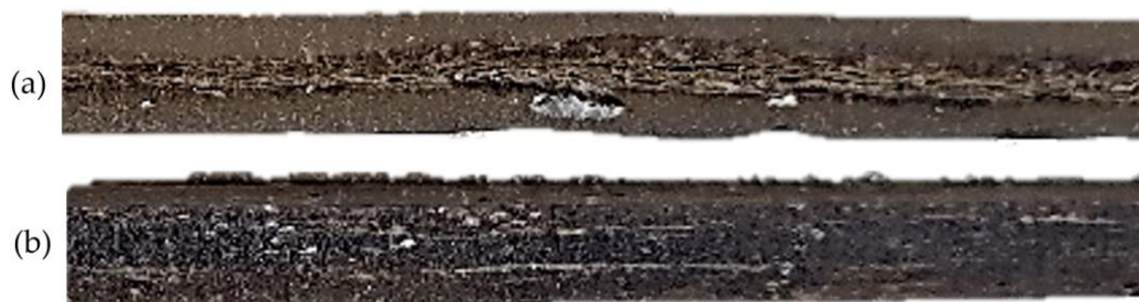
Figure 13. Comparison of specimens (side view) obtained by the sandwich method (a) and intermediate plate method (b) after testing.
