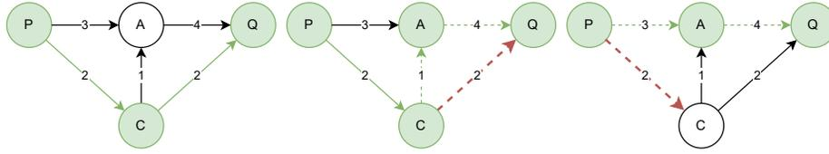
Fig. 1: Yen algorithm 3-shortest-paths (green paths) computation process between OD pair  $PQ$  based on the disconnection (red-dashed links) of each of the links forming the shortest path (green-lined path)
