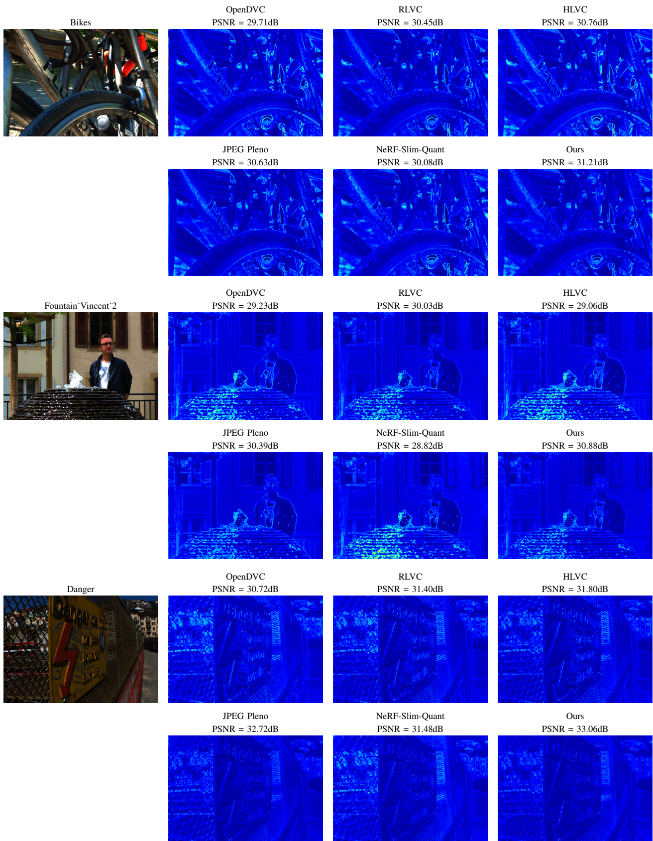
Fig. 4. The reconstruction error of the decompressed views obtained with PSNR-tuned models of OpenDVC, RLVC, HLVC and our method, as well as JPEG Pleno and NeRF-Slim-Quant. The bitrates are around 0.1 bpp.
