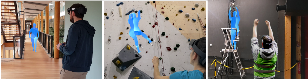
Figure 1: Control of self-avatars visualized through an Augmented Reality headset to better perceive interactions and affordances in the physical surroundings. Left Testing fire exit paths with a gamepad. Center Planning and testing a route before climbing by controlling the avatar’s limbs with gestures. Right Evaluating possible actions on a distant step stool with body-tracking mapping.
