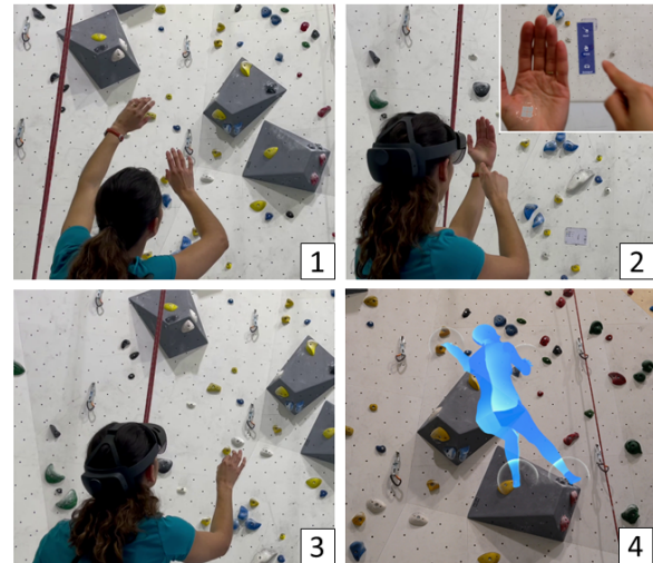
Figure 2: Example usage of our system. 1) A user is trying to figure out how to reach a hold on a boulder. 2) To better visualize her possibilities, she puts on an AR headset and launches the Puppeteering mode. 3) She then sets the position of her avatar with hand interactions. 4) The avatar as seen by the user (photo shot from the headset).
