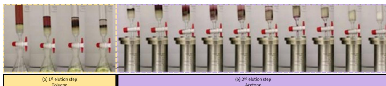
Figure 1. Photographs of the catalyst recycling protocol. (a) Migration of reaction products with toluene as eluting solvent (dark rhodium species stay at the top of the column), (b) Migration of the dark rhodium species with acetone as eluting solvent, with total silica column discolouration and direct recovery in the autoclave reactor.
