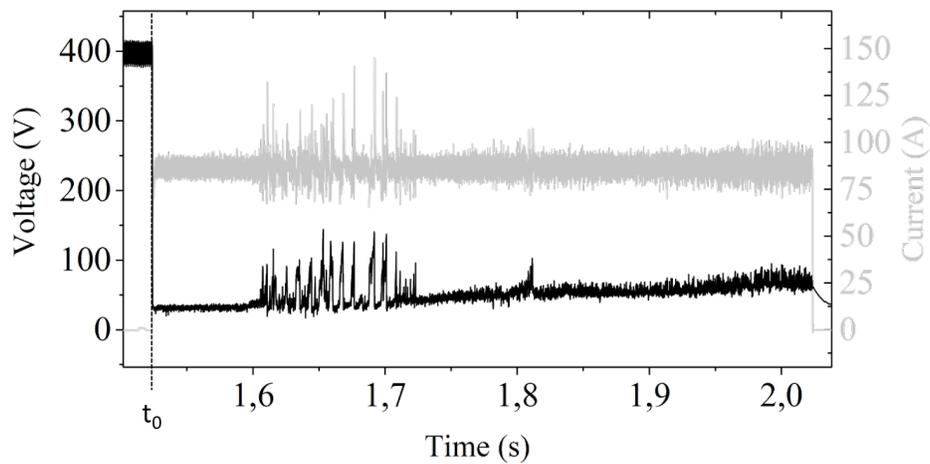
Figure 6: Typical arc current and voltage in DC.
