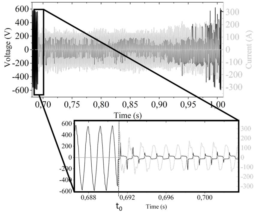
Figure 5: Typical arc current and voltage in AC.
