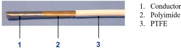
Figure 3: Composition of the aluminium and copper cables used in this work.
