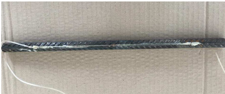
Fig. 1. Picture of the steel rebar of \varnothing 12 mm, showing the OF sealed in the engraved groove
