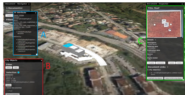
Figure 8. Contextual view of a building of a slab constructed using : a spatial representation as 3D geometry in blue from an Ifc file, and thematic information coming from an Ifc file (in frame A), the geometry (in frame B), documents (in frame C)
