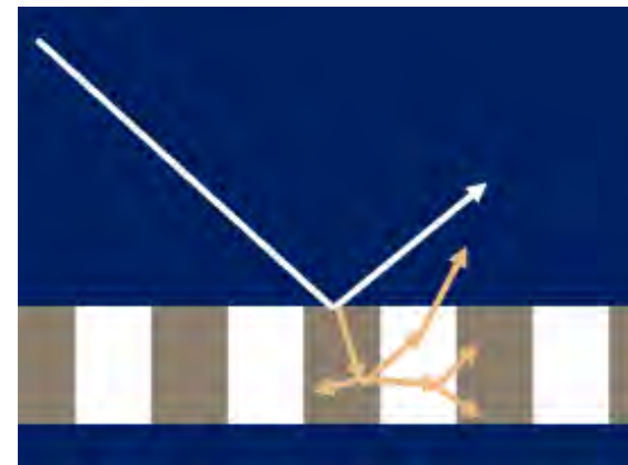
Diffusion of light inside the substrate
