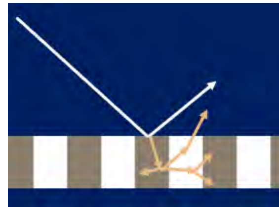
Diffusion of light inside the substrate
