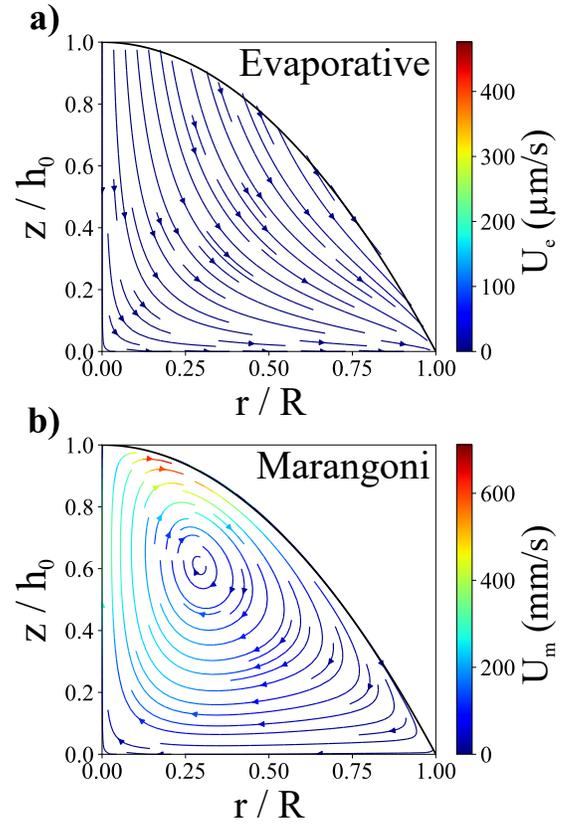
Fig. 5 Numerical streamlines of the evaporative (a) and of the Marangoni (b) flows for  $\Delta T_m = 20 \text{ K}$ ,  $\sigma = 350 \mu\text{m}$ ,  $R = 1 \text{ mm}$ ,  $t_f = 40 \text{ s}$  and  $h_0 = 176 \mu\text{m}$ .
