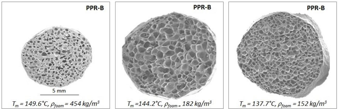
*Figure 7: Foam structure of the foamed extrudates for PPR-B.*
