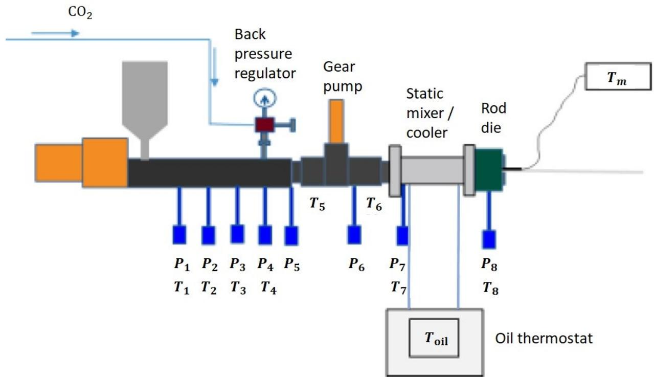
Figure 3: Physical foaming extrusion disposal. The sensors for temperature and pressure measurements are indicated.
