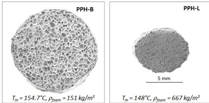
*Figure 8: Foam structure of the foamed extrudates for PPH-B and PPH-L grades.*
