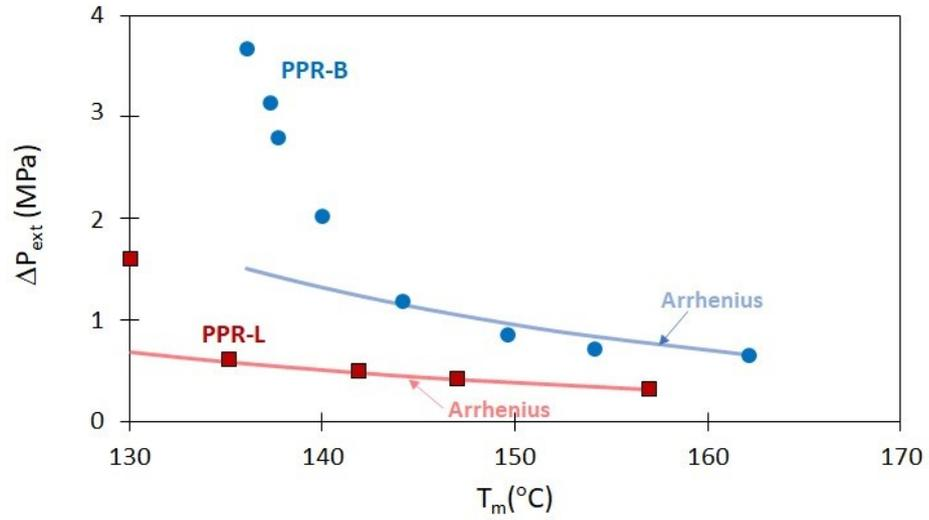
Figure 10:  $\Delta P_{ext}$  as a function of temperature for branched (circular symbols) and linear (square symbols) PPR grades. Continuous lines represent the respective Arrhenius thermal dependence of  $\Delta P_{ext}$  starting from the largest melting temperature in absence of crystallization using the activation energy determined under shear.
