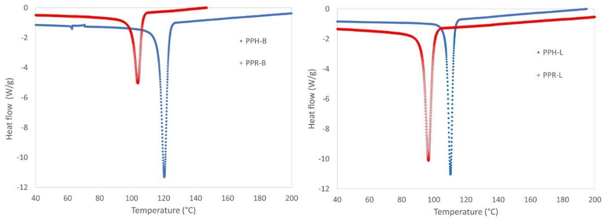
*Figure A: Crystallization curves for branched grades on the left, for linear grades on the right.*
