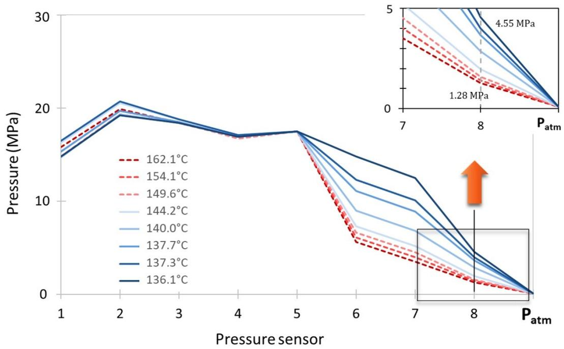
Figure 5: Pressure profile as a function of the foaming temperature  $T_m$  (PPR-B).
