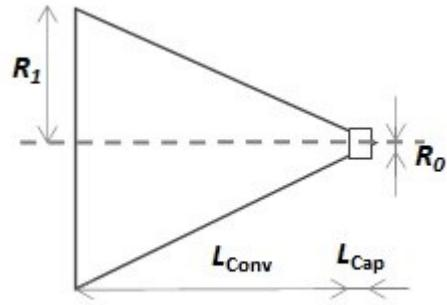
Figure 4: Schematic drawing of the extrusion die geometry.
