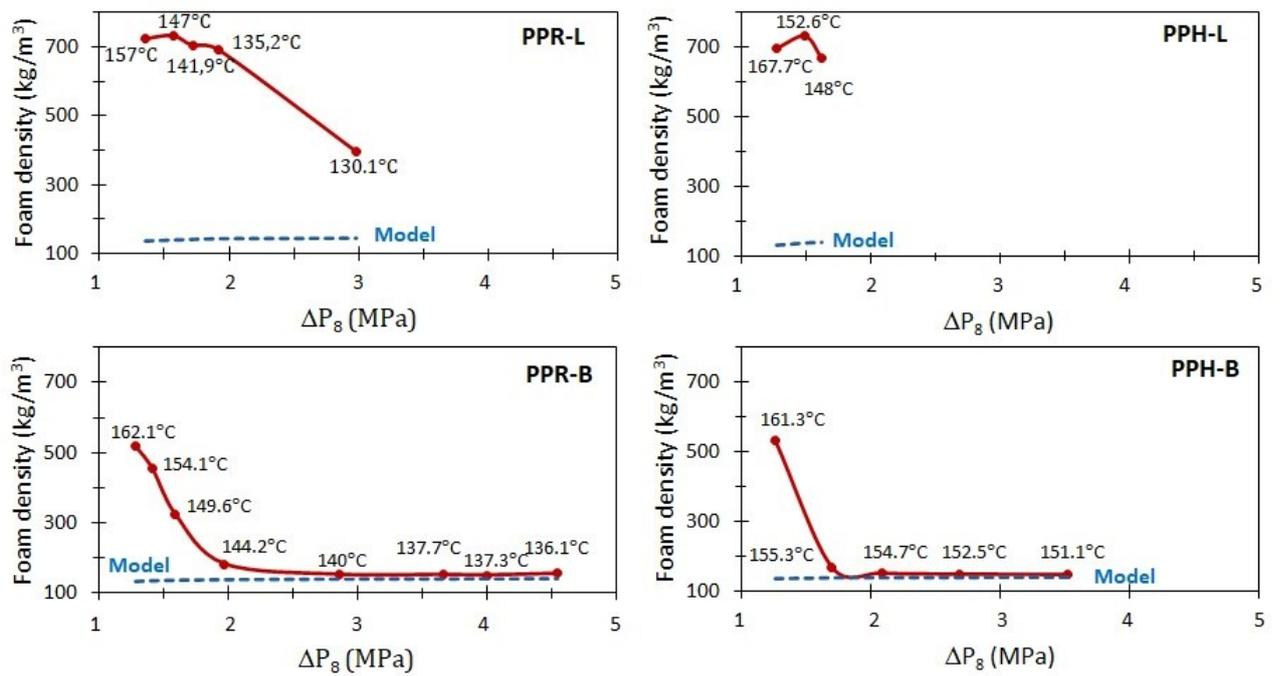
Figure 6: Relationship between foam density and pressure drop in the die for the four linear and branched polypropylenes. Dashed lines correspond to the theoretical density (Eq. 9).
