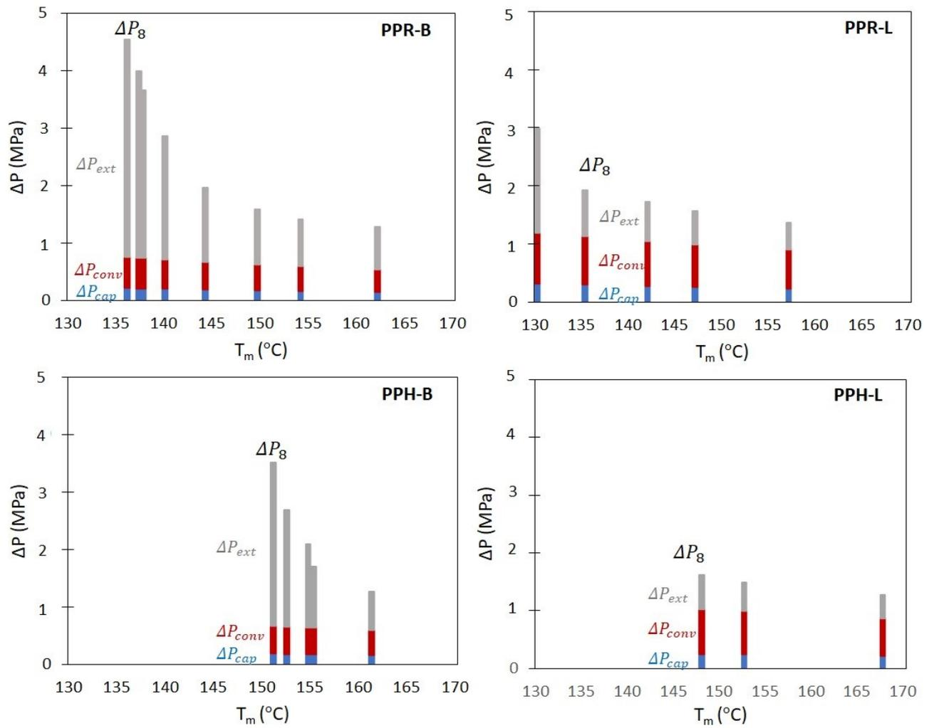
Figure 9: Comparison between the measured pressure drop  $\Delta P_8$  and the calculated pressure drop in the capillary  $\Delta P_{cap}$  and in the convergent  $\Delta P_{conv}$  for the four grades.
