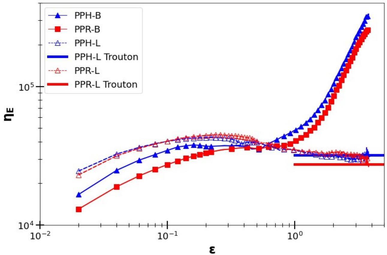
Figure 2: Elongational rheology versus strain  $\epsilon$  for the different PP grades at  $170^\circ\text{C}$  and  $\dot{\epsilon} = 0.1 \text{ s}^{-1}$ . Troutonian viscosities (calculated from shear viscosities) of the linear grades were indicated for sake of comparison with the steady state elongational viscosities.
