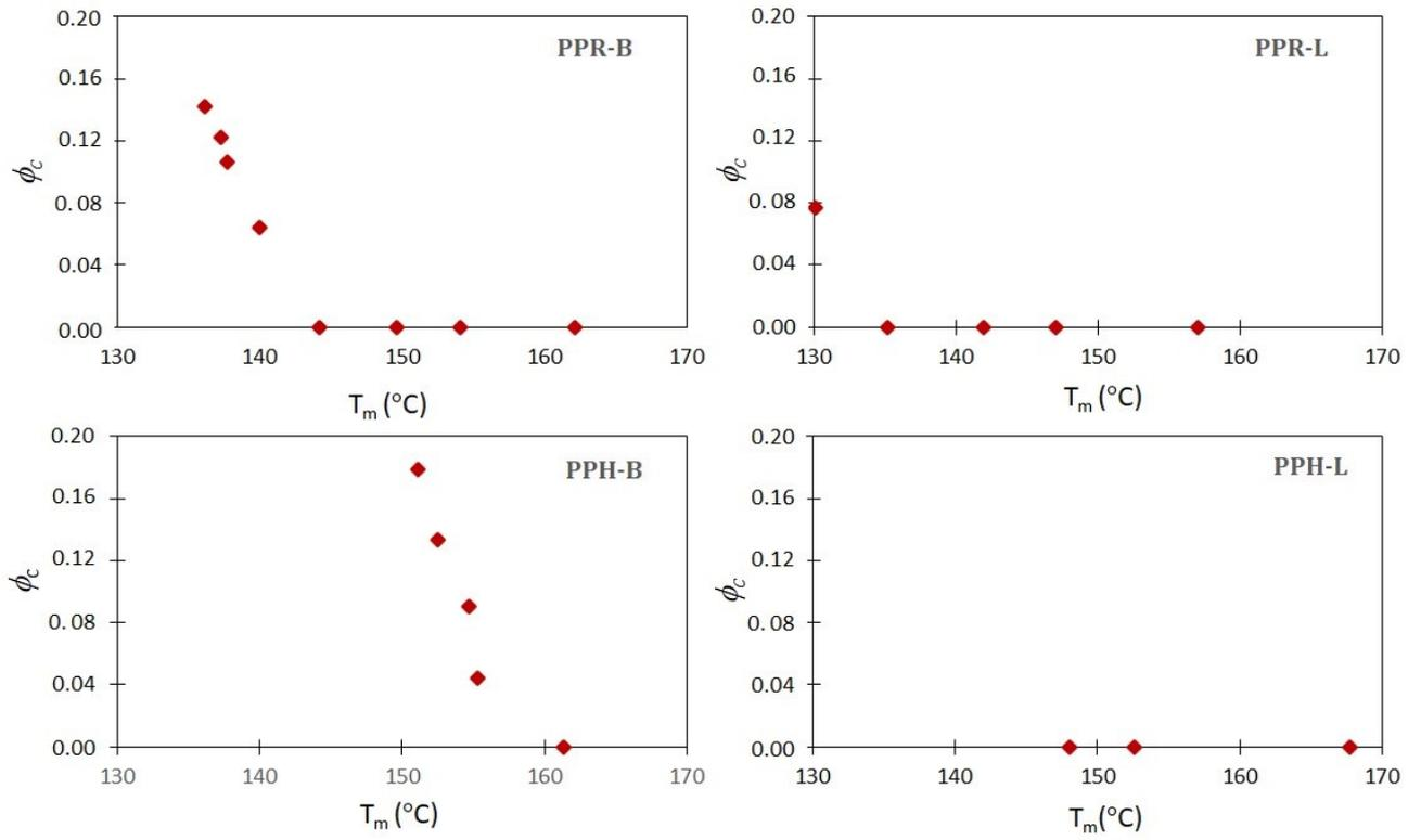
*Figure 11: Calculated crystallized volume fraction as a function of foaming temperature for the different polypropylenes*
