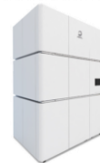
HRTEM JEOL 300 keV low dose for ultra-high resolution and sensitive materials (organic - perovskite) Liquid/Electrical/temperature holder Poseidon for operando Solid/Liquid and solid/gas interface 4D-STEM, 3DED Tomography (In lab ready by end 2022)
