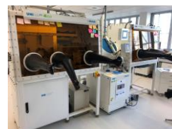
Ar-filled glovebox for PSC fabrication including spin coaters and two sources with organic thermal evaporator (Mbraun)
