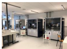
X-ray diffraction Bruker D8 Advanced Reflection and transmission with rotating anodes In situ with and in combination with Temperature, humidity, atmosphere, electrical bias, light
