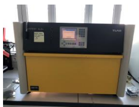
Light soaking chamber for accelerated ageing tests IEC61646
