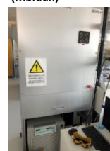
Light soaking chamber for accelerated ageing tests for modules IEC61646
