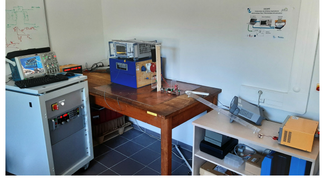
Fig. 8. EMC measurement setup with introduced all precautions.
