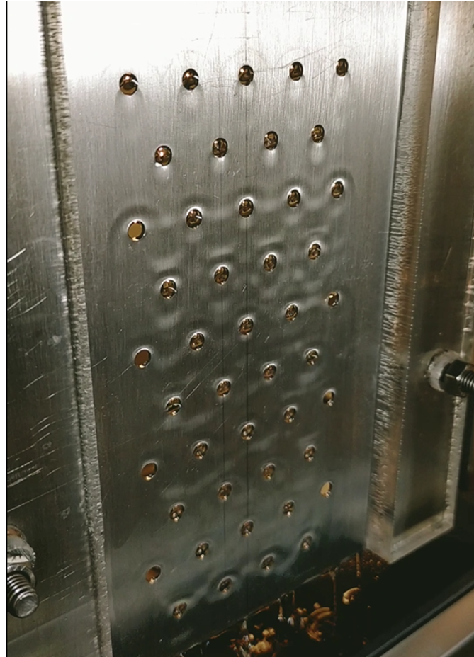
Figure S10. Liquid film pattern on a staggered array of perforations at Re = 35 \cong Re_{cr} when all perforations are in curtain mode. Plate thickness t = 1 mm, perforation diameter d = 4 mm and spacing s = 14 mm. Full view of the back of the plate.
