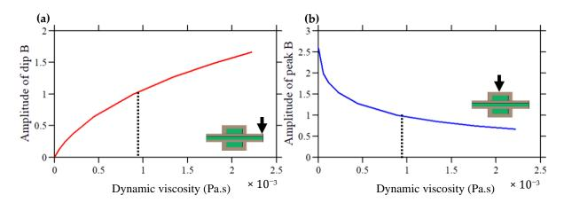
**Figure 6.** Amplitude of mode B of the washer as a function of the dynamic viscosity of the liquid, evaluated from (**a**) the transmission and (**b**) the surface of the washer. The dotted line indicates the value of the dynamic viscosity of the water ( $\mu = 8.9 \times 10^{-4} \text{ Pa} \cdot \text{s}$ ). The curves are normalized to their values at the water's viscosity.
