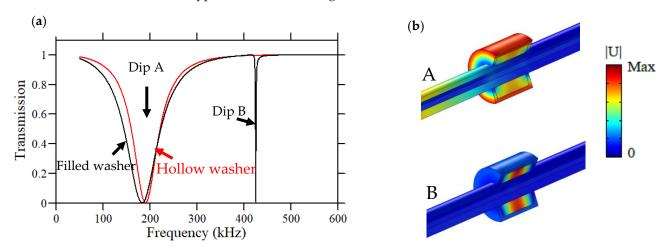
**Figure 2.** (a) Transmission curves of the acoustic liquid sensor when the washer is filled with water (black curve) and when it is empty (red curve). (b) Maps of the displacement fields of dips A and B.
