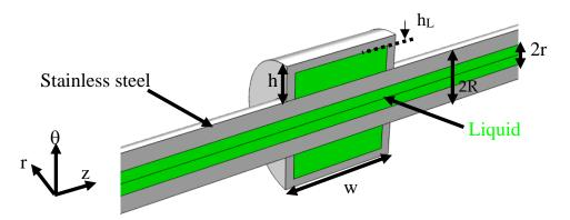
**Figure 1.** 2D cross-section view of the acoustic liquid sensor composed of a hollow cylindrical washer surrounding a hollow tube. The green and grey parts, respectively, represent the liquid and solid materials.
