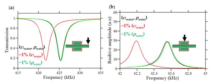
**Figure 4.** Transmission curves of the acoustic liquid sensor evaluated on (**a**) the transmission region and (**b**) the washer. The black curve corresponds to water, while the red and the green curves correspond to a change of 1% in the sound velocity  $c_l$  and the mass density  $\rho$  of the water, respectively.
