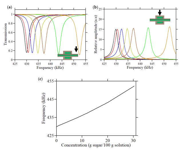
**Figure 5.** (a) Transmission curves calculated for a set of sucrose concentrations in an aqueous sugar solution, with (b) the same as (a) for a measurement on the surface of the washer. (c) Dip frequencies as functions of the associated sugar concentration.
